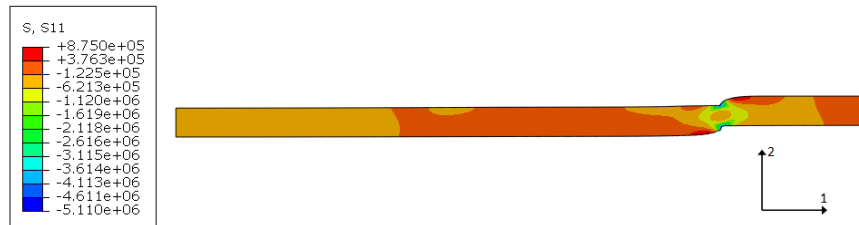
Figure 3.15: Radial stress of 8-layer panel with supported punch (Pa).
