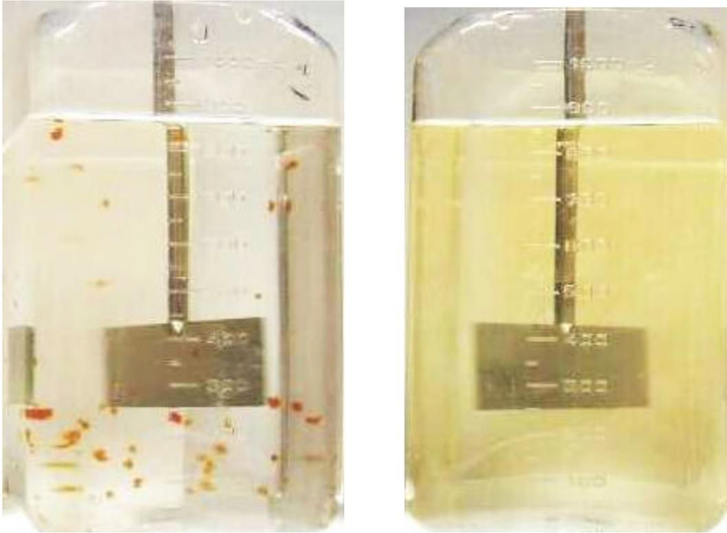
**Figure 1-7. Groundwater conventional sedimentation flocs with addition of 0.2 mg/L polymer (left) and no polymer (right).**
