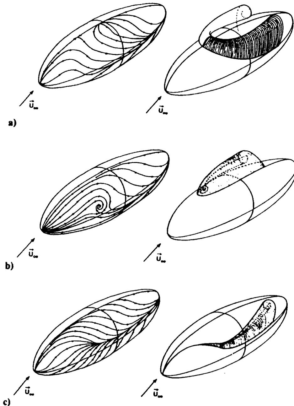
Figure 1.1: Limiting streamline pattern and surfaces of separation for three types of 3-D separation: (a) horseshoe type separation; (b) Werle type separation (the view of the surface separation is rotated  $90^\circ$  from the view of the limiting streamline pattern); (c) cross flow separation. Taken from Yates and Chapman [1].
