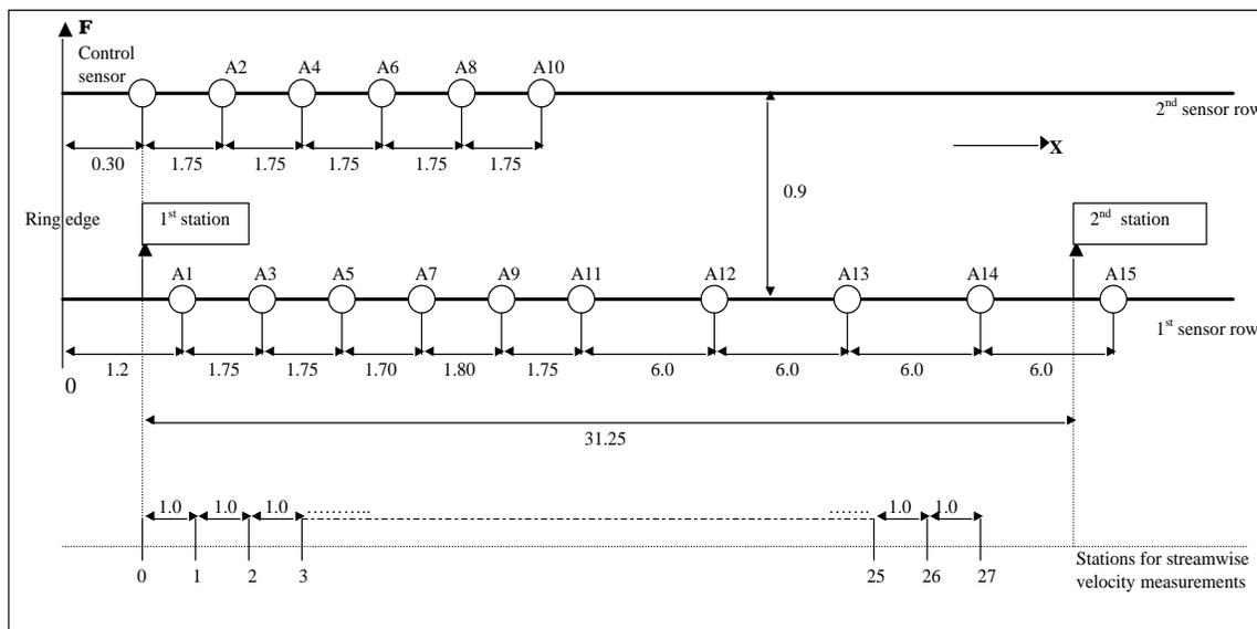
Figure 4.4: Planform view of the sensor configuration, boundary layer traverse and streamwise velocity measurement stations (all dimensions are measured in inches and the figure is not drawn to scale).
