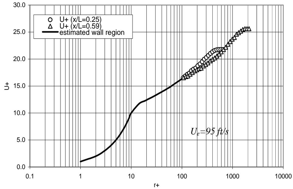
Figure 4.6: Boundary layer velocity profiles for  $U_e = 95$  ft/s.
