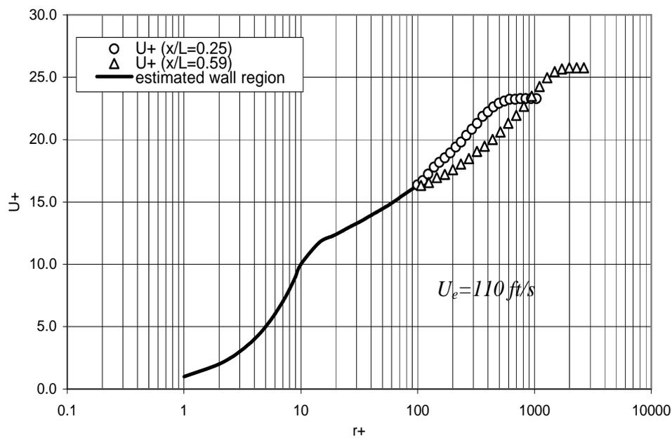
Figure 4.7: Boundary layer velocity profiles for  $U_e = 110 \text{ ft/s}$ .
