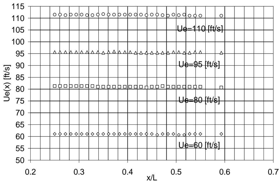
Figure 4.8: Streamwise Velocity Distributions for all calibration speeds.
