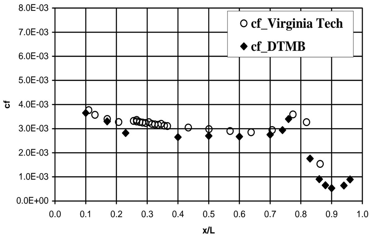
Figure 4.9:  $C_f$  vs.  $x/L$  at  $0^\circ$  angle of attack (For the measurements at Virginia Tech  $Re_L = 5.5 \times 10^6$ , for the measurements at David Taylor Model Basin (DTMB)  $Re_L = 1.2 \times 10^7$ )
