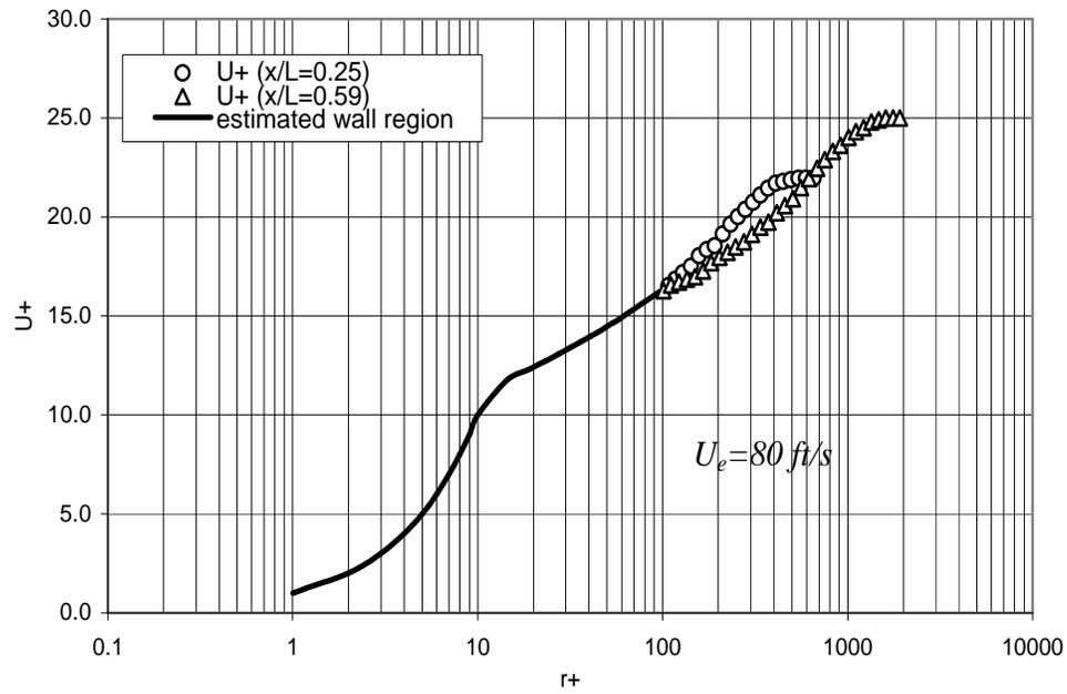
Figure 4.5: Boundary layer velocity profiles for  $U_e = 80$  ft/s.
