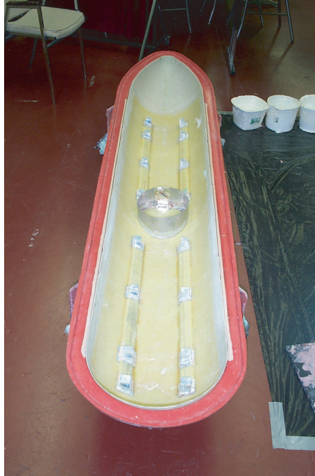
Figure 45: Half of the hull in the female mold
