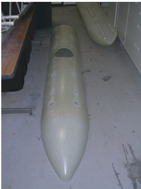
Figure 44: Top half of the hull constructed of fiberglass
