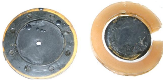
Figure 3-12: Metal-elastic mount that failed under high amplitude testing.
