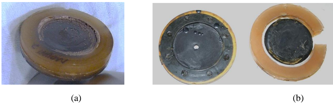
Figure 4-20: Failed Mount from BM Southern's Quasi-Static Test [11](a) and failed mount from the dynamic test in this study (b)
