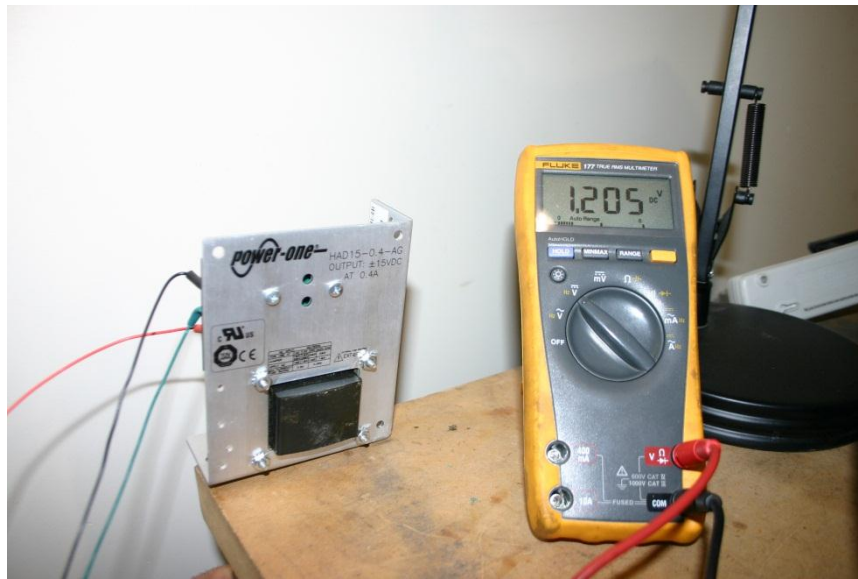
Figure 3-9: LVDT Power supply (left) and multi-meter (right).
