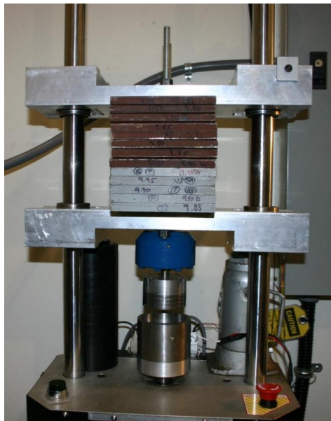
Figure 3-19: Finalized completed assembly with rheometer, load cell and weights between the braces all mounted on the EMA.
