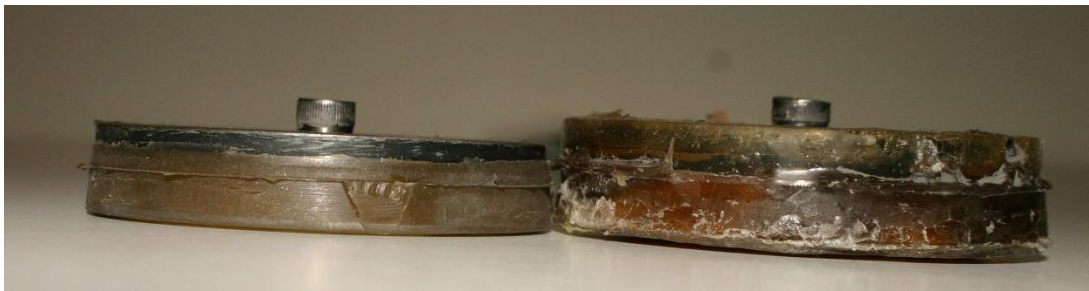
Figure 3-13: Original MRE mount (left) and modified MRE mount (right).
