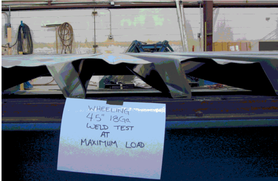
Figure 4-13: Warping distortion of N-Deck
