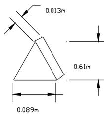
Figure 2.5 Shape and dimension of small spires used for configuration #3
