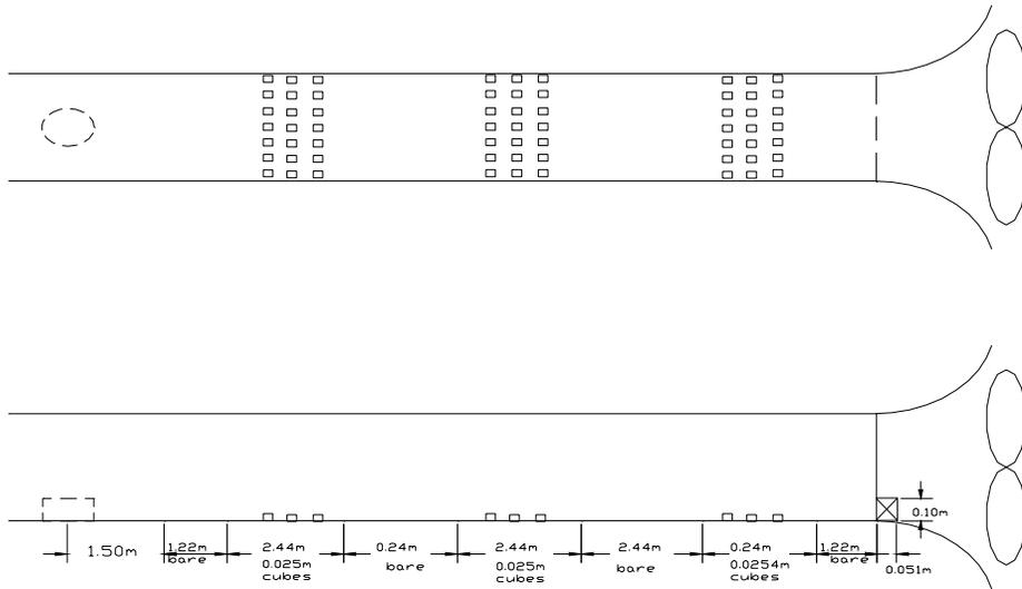
Figure 2.8 Trip dimensions, and roughness locations used for configuration #6
