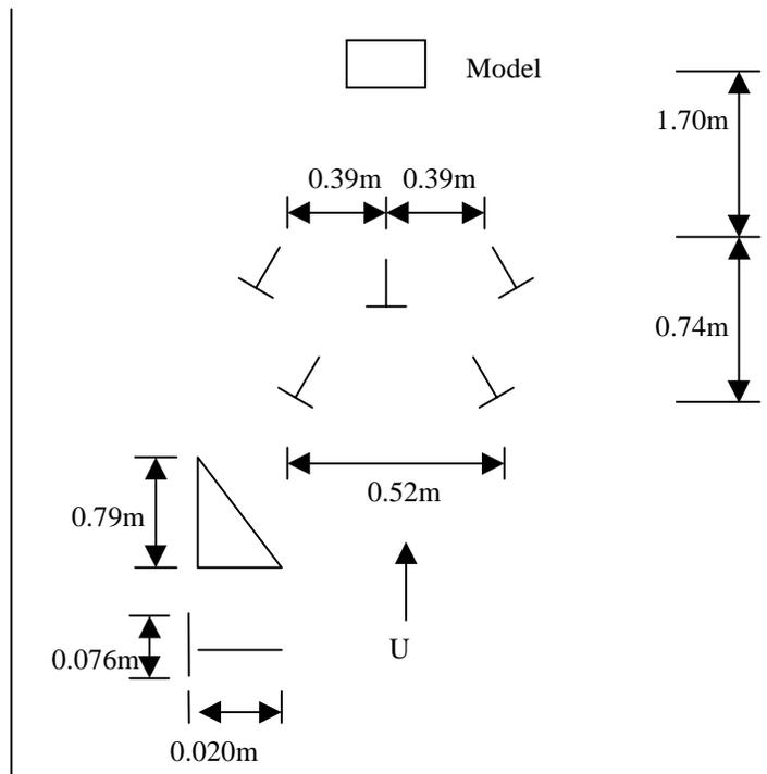
Figure 2.9 Placement of spires for configuration #7
