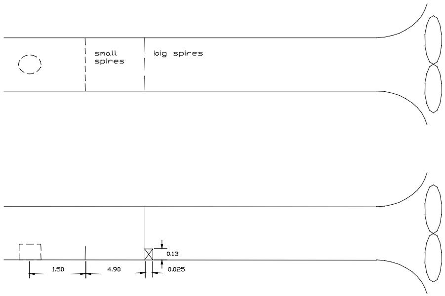
Figure 2.10 Trip dimensions and spires locations used for configuration #8
