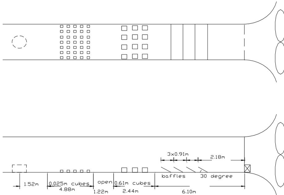
Figure 2.6 Dimensions, placement locations and characteristics of roughness elements used for configuration #4
