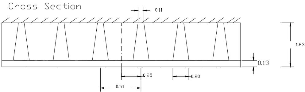
Figure 2.11 Dimensions, placement locations of small spires used for configuration #8
