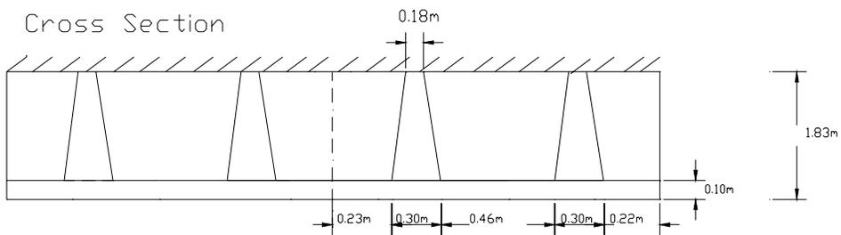
Figure 2.7 Dimensions and placement locations of large spires used for Configuration #6
