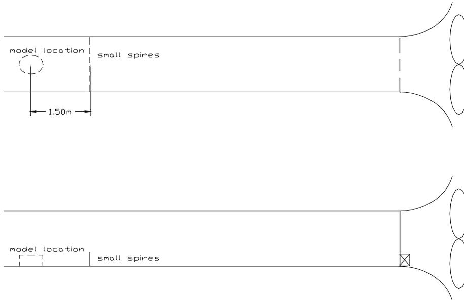
Figure 2.3 Trip and spires locations for configuration #3
