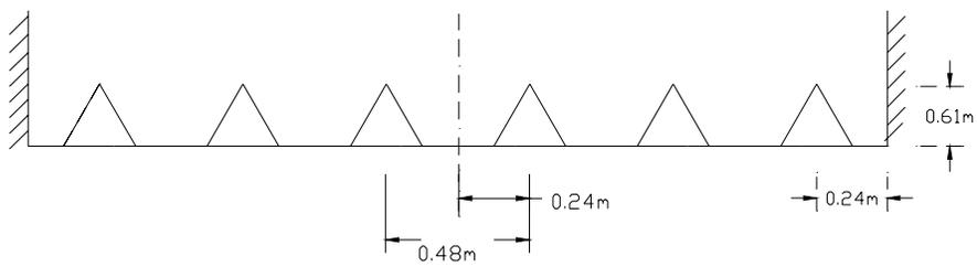
Figure 2.4 Placement locations of the six small spires for configuration #3
