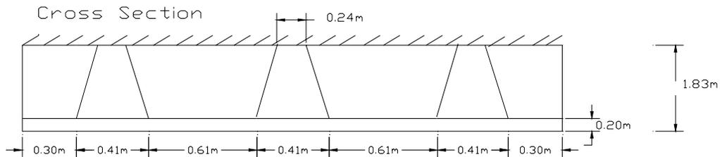
Figure 2.2 Cross-Section of big spires placed at tunnel entrance for configuration #2
