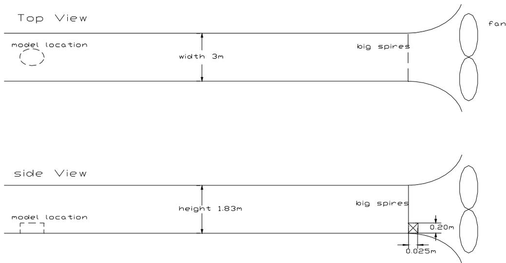
Figure 2.1 Plan and Side views of the Clemson tunnel for configuration #2
