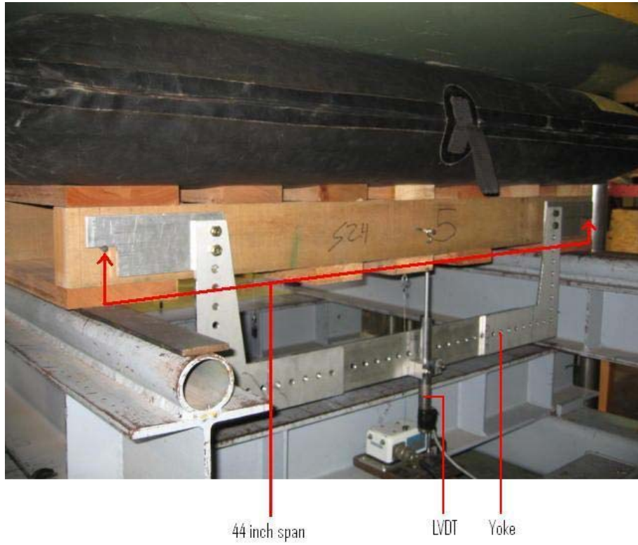
Figure 12: Photograph showing the LVDT/Yoke set up for a RAL bending test.
