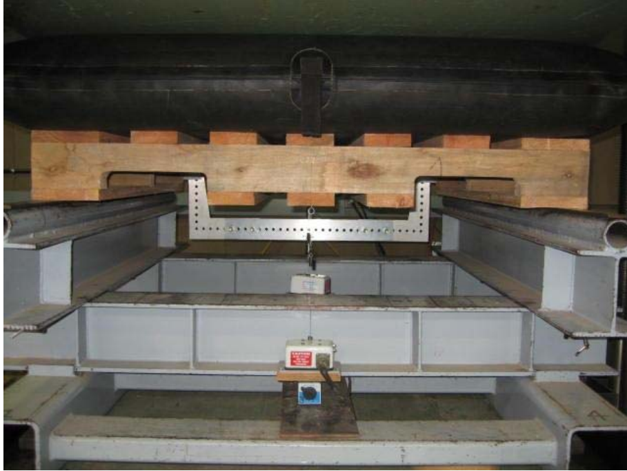
Figure 18: Photograph showing the RAL test set up for a notched heavy duty pallet.
