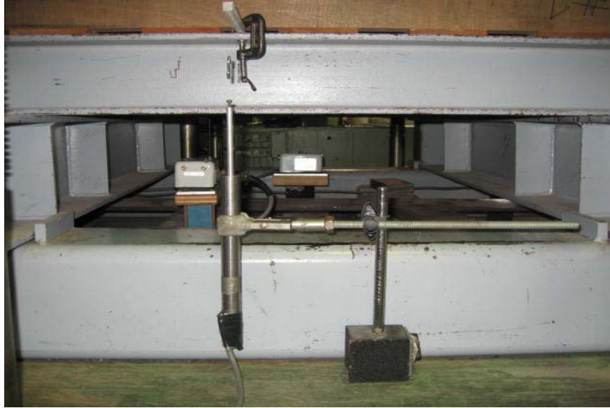
Figure 19: LVDT set up for light duty pallet floor stack tests.
