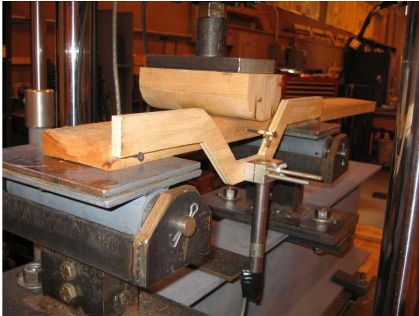
Figure 1: Picture showing single point bending test for deck board MOE.
