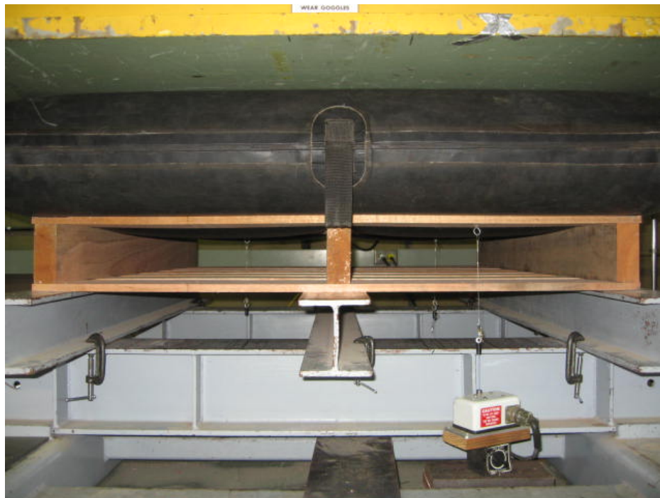
Figure 21: Photograph showing the set up for a light duty 3 stringer bottom deck floor stack bending test.
