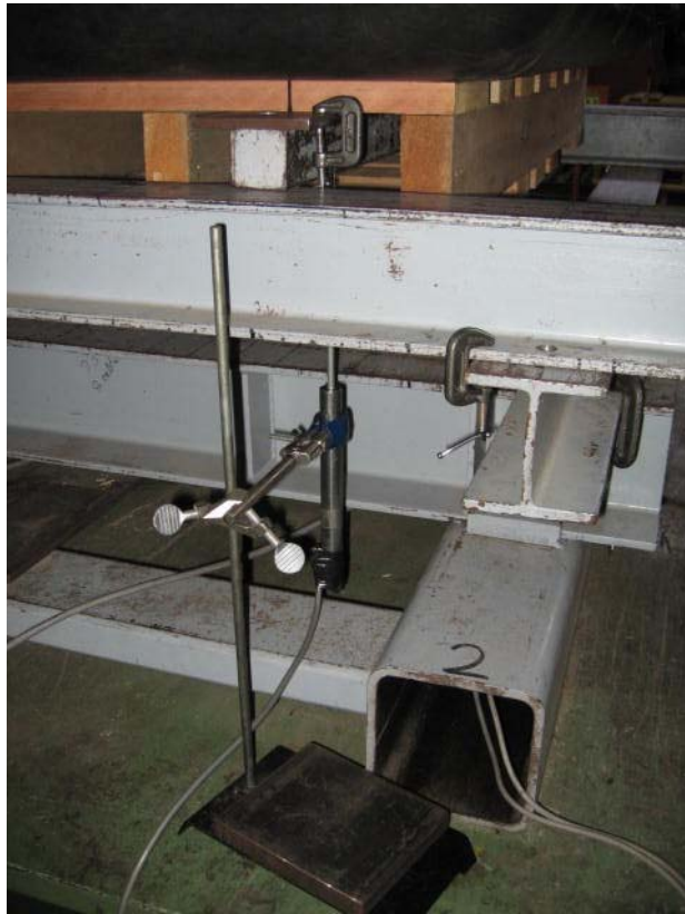
Figure 14: Photograph showing the LVDT set up for non-notched fork tine support bending tests.
