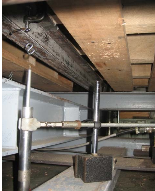
Figure 20: Photograph showing the LVDT set up for a notched heavy duty fork tine support bending test.
