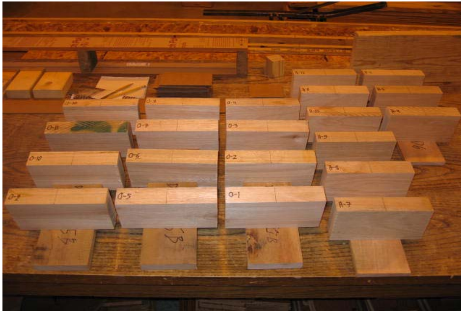
Figure 33: Photograph showing the joint withdrawal test specimens.
