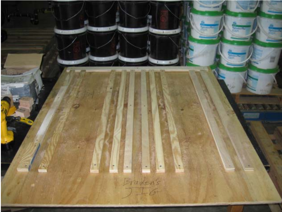
Figure 8: Photograph showing the pallet assembly jig.
