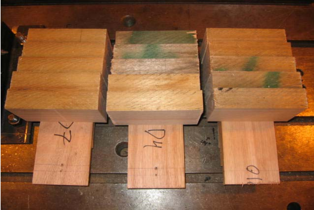
Figure 29: Photograph of stacked joint rotation samples.
