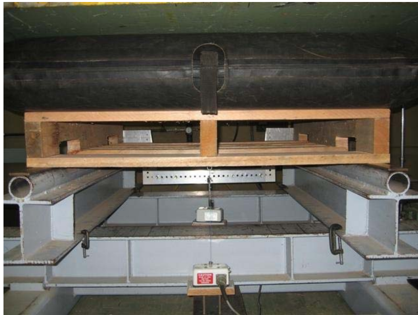
Figure 19: Photograph showing the RAW test set up for a notched heavy duty pallet.
