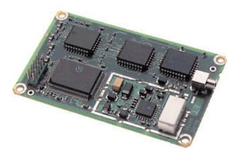
Figure 3.8 – Motorola VP Oncore GPS Receiver (from Motorola Oncore User's Guide)
