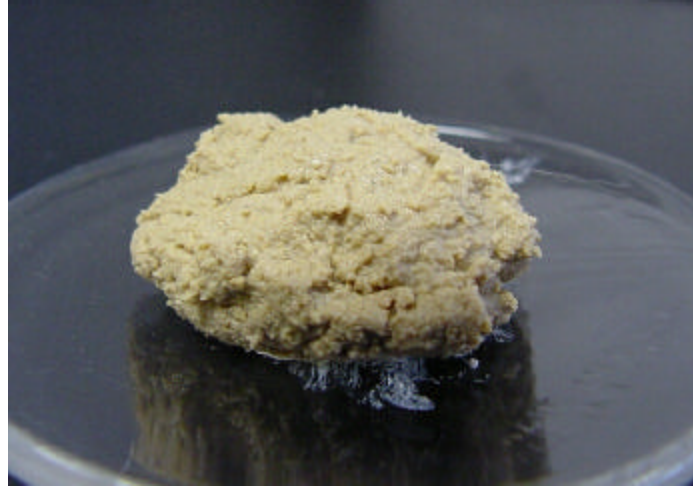
Figure 1-2) Sample of deposited solids from Denver distribution system
