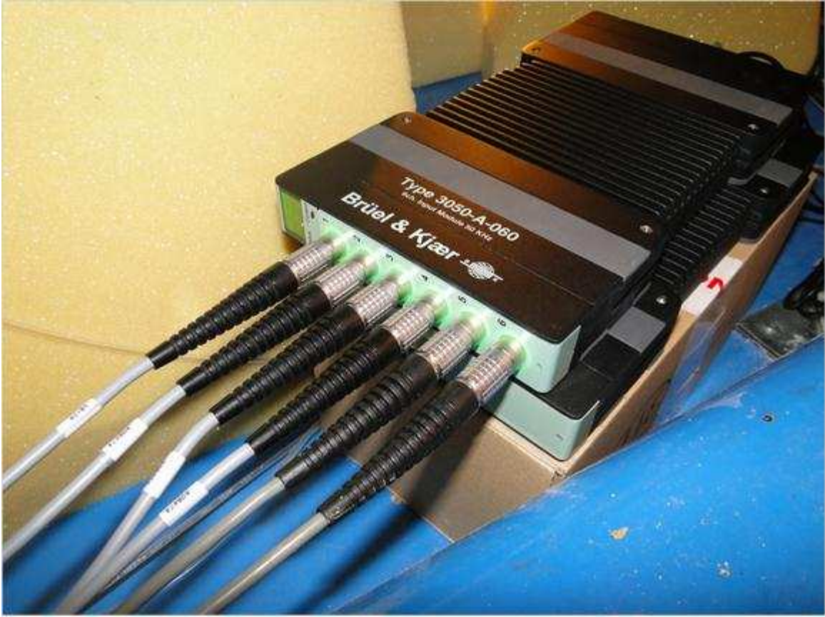
Figure 18. LAN XI data acquisition hardware
