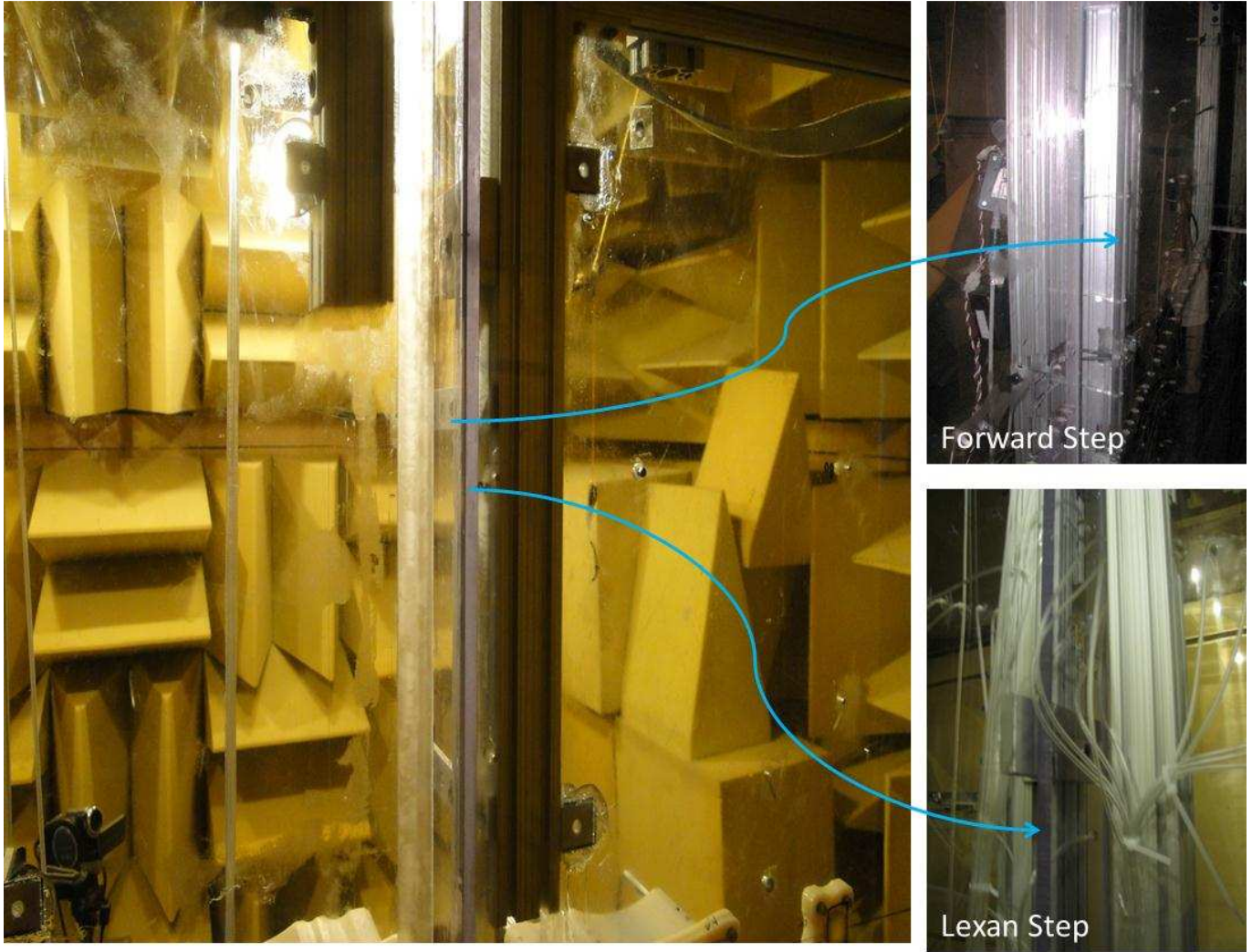
Figure 9. Forward step in position inside test section
