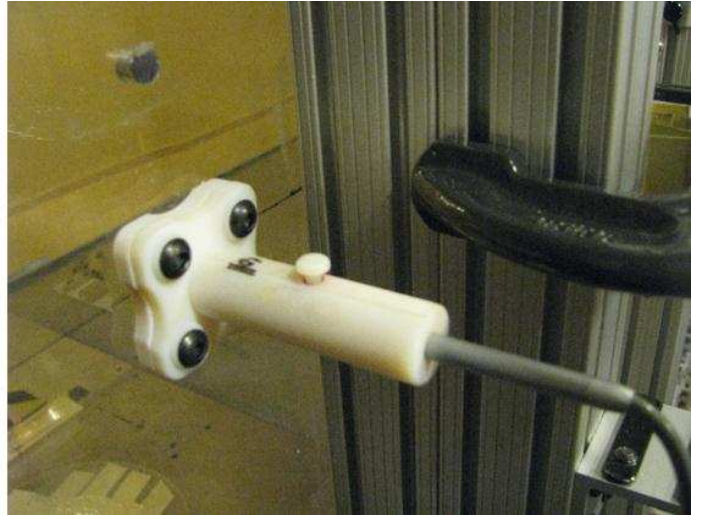
Figure 13. Rear view of the microphone holders
