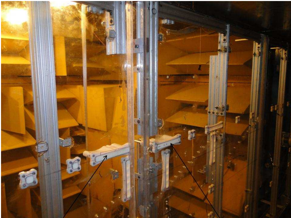
Figure 13. Rear view of the microphone holders
