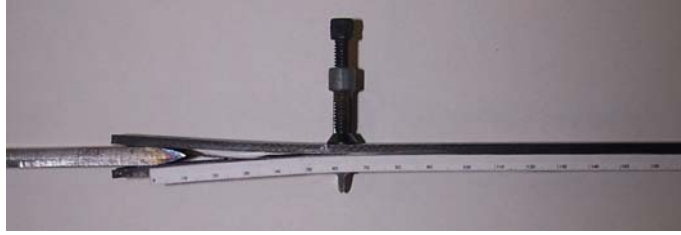
Figure 3.3. Specimen pre-cracking procedure.
