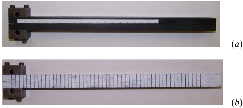
Figure 3.4. Typical bonded composite specimen configurations prior to testing: (a) static and (b) dynamic.
