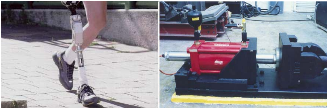
Figure 2-4. Prosthetic MR damper and 180 kN double-ended MR damper for civil engineering applications [19]
