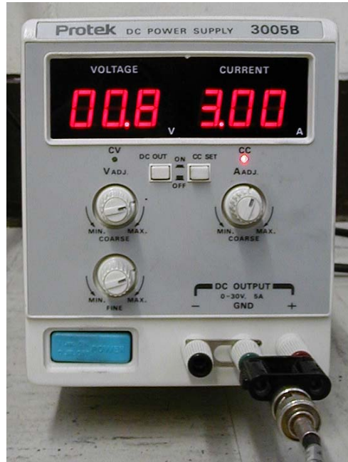
Figure 4–2. Protek 3005B DC Power Supply for providing current to MR dampers
