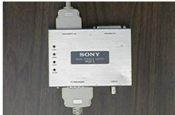
Figure 3–10. PCIF-5 interface for controlling and transferring data to computer
