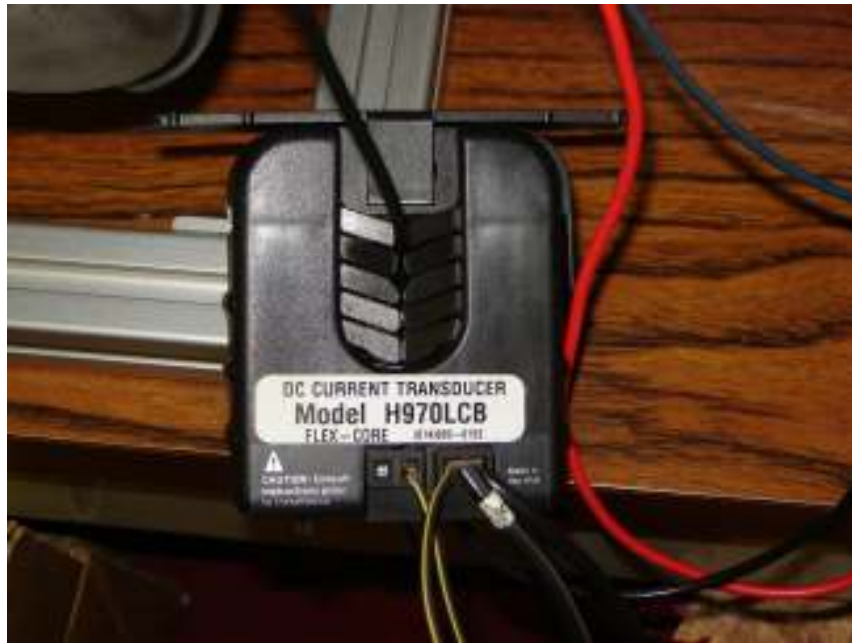
Figure 11. Current transducers are used to measure the current flowing through the motors from the motor controller PWM signal.
