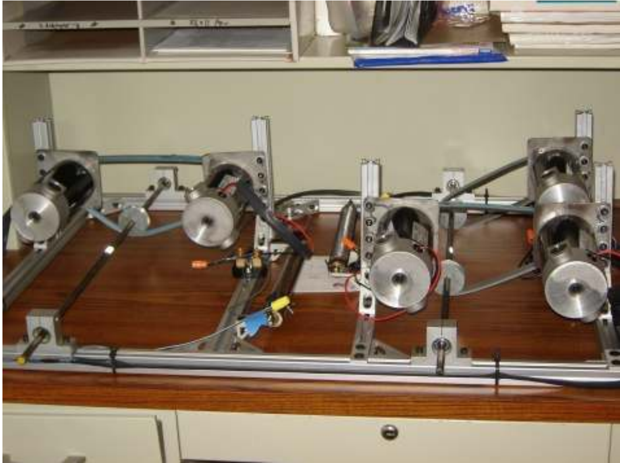
Figure 9. T-SLOTS aluminum extrusion was used as a frame for the system
