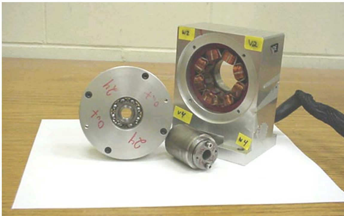
Figure 2.5: Radial magnetic bearing disassembled showing the radial rotor the stator and the back-up bearing
