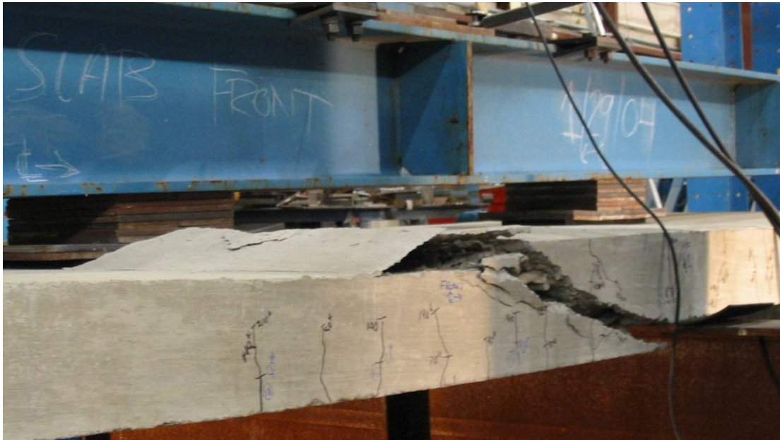
Figure 4.44 - Shear failure of the Strength 2 specimen
