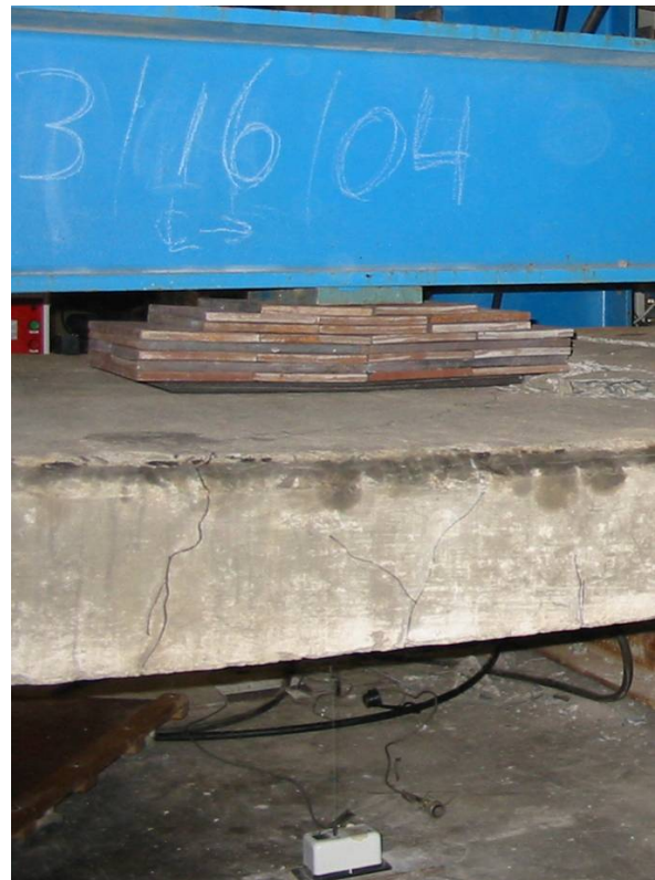
Figure 3.18 - Load point setup and wirepot (post failure - weigh station deck)
