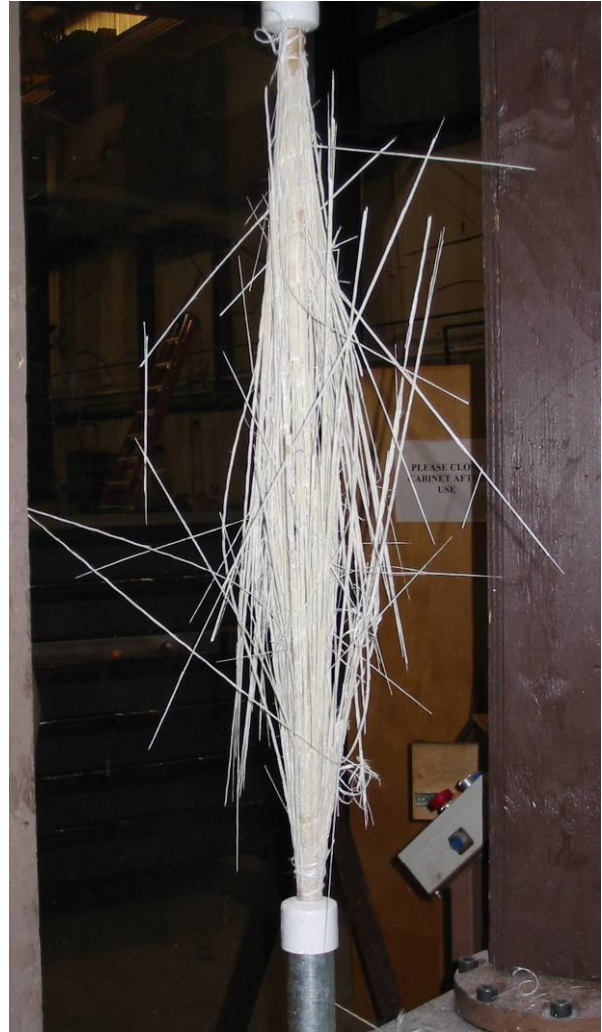
Figure 3.23 - Typical GFRP tensile test failure
