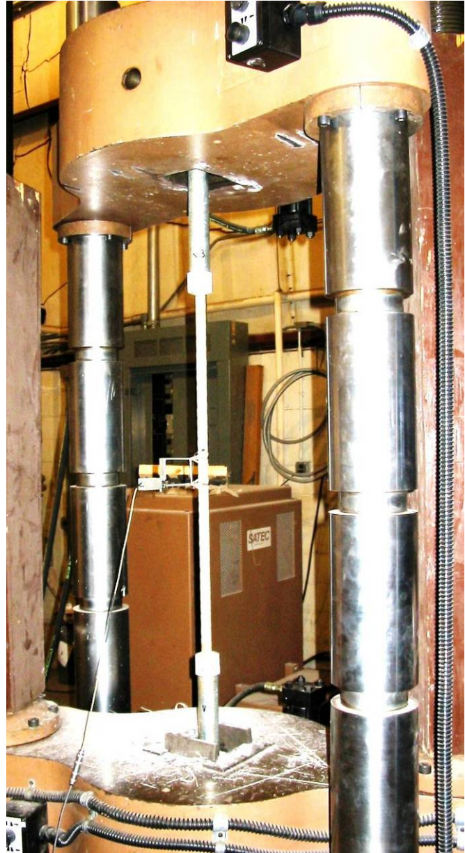
Figure 3.22 - Tensile test setup
