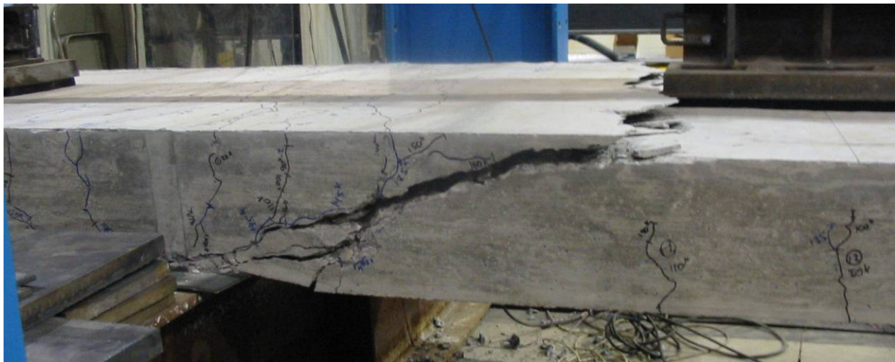
Figure 4.4 - Shear failure of the 3.5 ft shear specimen
