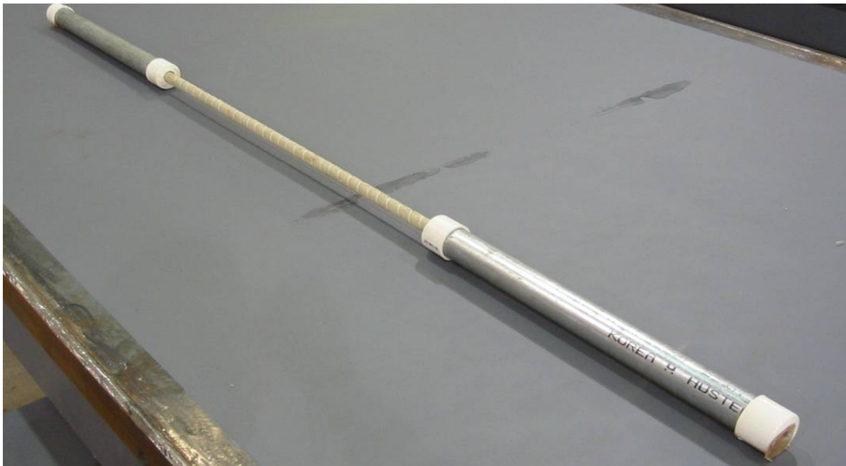
Figure 3.21 - Typical GFRP bar tensile test specimen with end anchors
