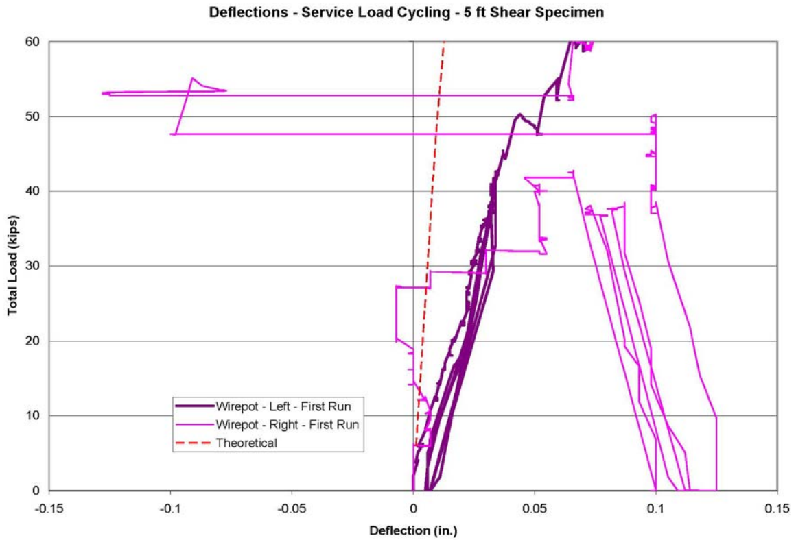
Figure H.8 – Deflection plot for the 5 ft shear specimen during service load cycling
