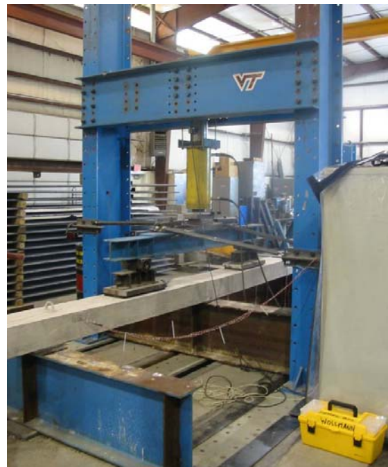
Figure 3.4 - Lab setup with the 1 ft deck
