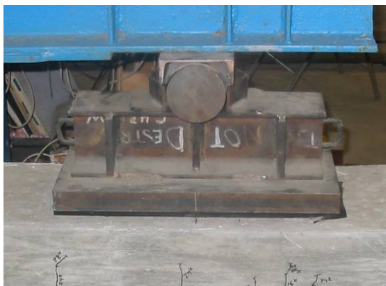
Figure 3.6 - Point load setup for the 1 ft deck
