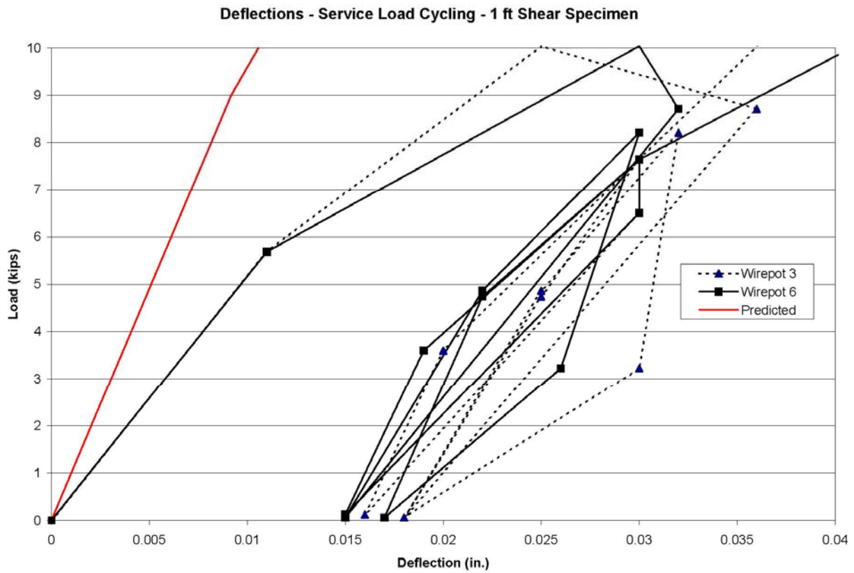
Figure 4.10 - Plot of load versus deflection during the service load cycling of the 1 ft shear specimen
