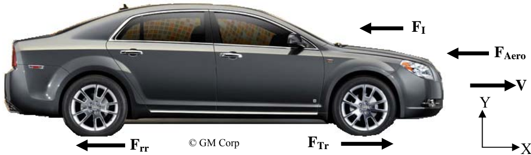
Figure 3. Force balance on 2008 Chevrolet Malibu.
