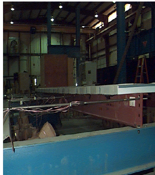
Figure 2.6 Instrumented Rods Used as Load Cells
