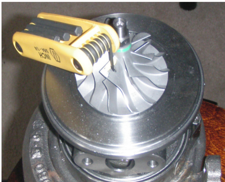
Figure 2.14. Compressor wheel with allen key resting in an installed set screw.
