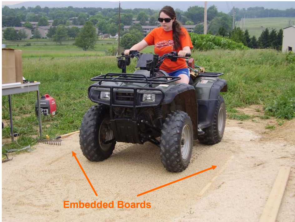
Figure 6-11: Embedded Boards Used in Sand Pits in Spring/Summer 2007 Tests
