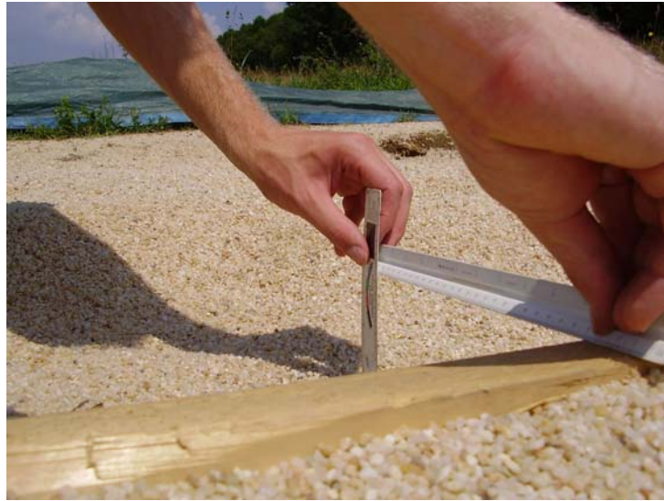
Figure 6-4: Sinkage Measurement Technique Employed in Spring/Summer 2007 Tests
