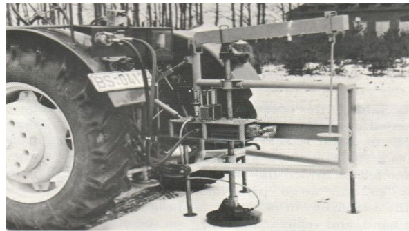
Figure 2-1: Vehicle-Mounted Bekker's Values Meter (Bevameter) in Use on Snow [3]
