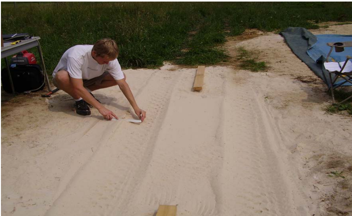
Figure 6-17: Sinkage Measurement Procedure for Spring/Summer 2007 Data Collection
