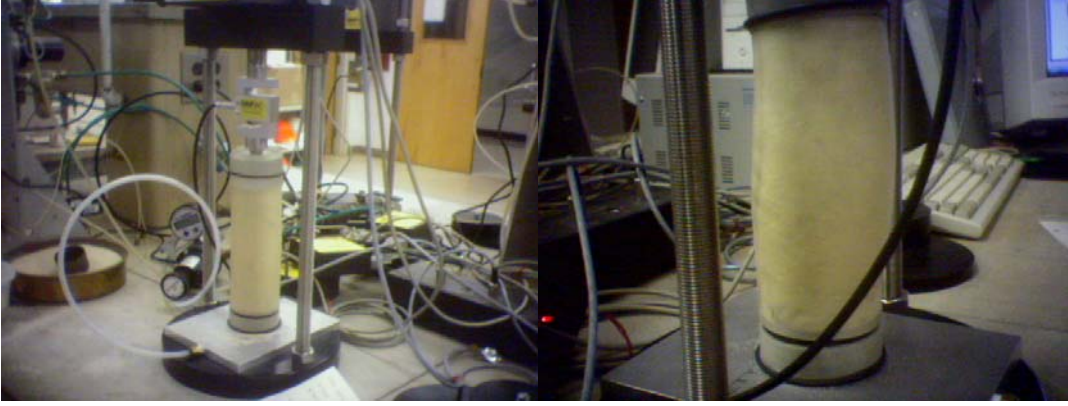
Figure 2-5: Triaxial Shear Test (a) Apparatus and (b) Failure Mode
