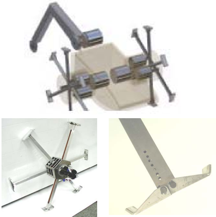
Figure 4-3: IMPASS Virtual Model, Spoke-Wheel Prototype and Foot
