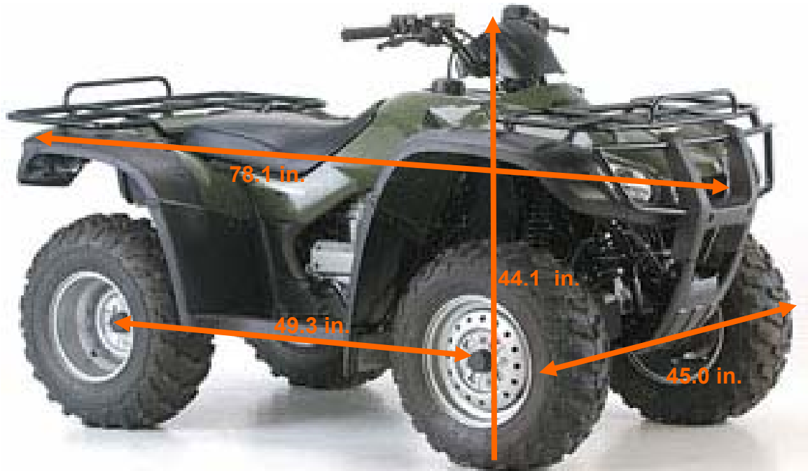
Figure 5-3: 2004 Honda ATV used in Spring/Summer 2007 Tests [31]
