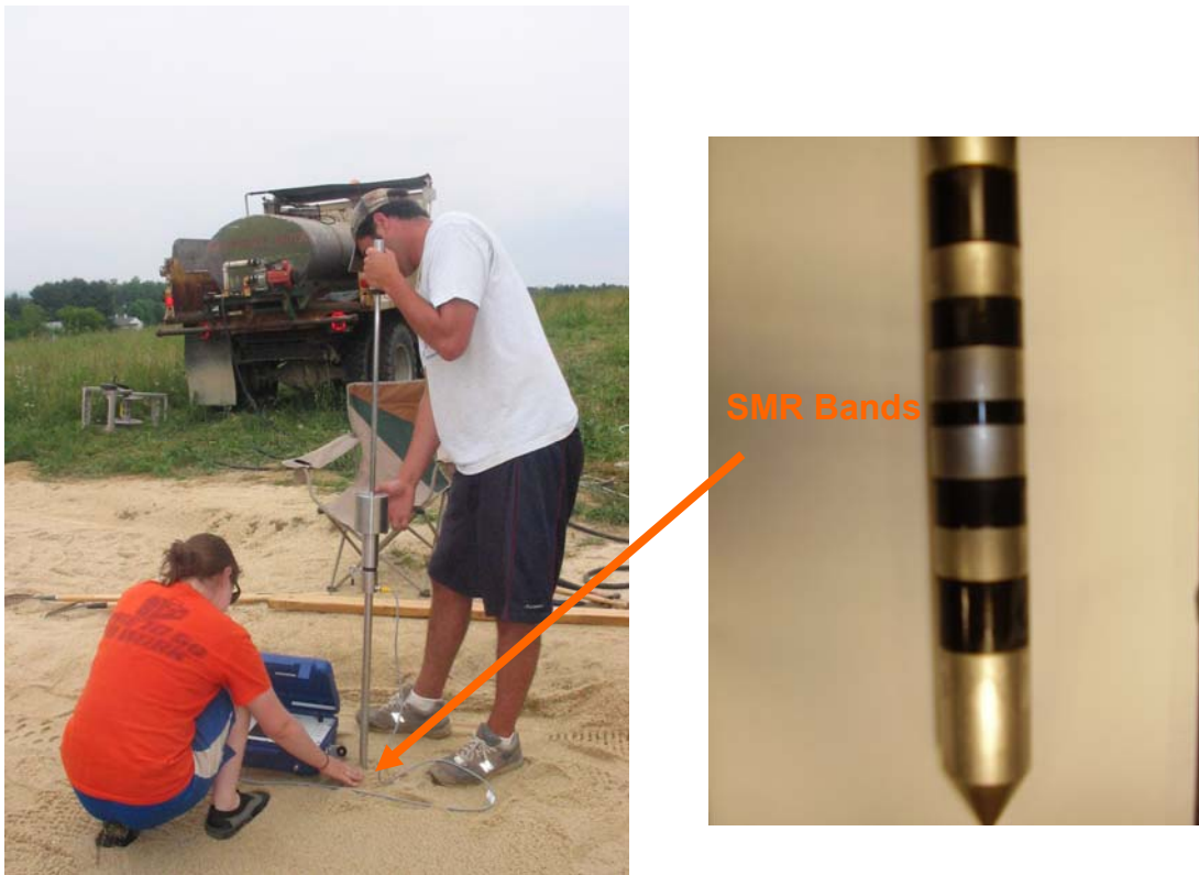
Figure 6-3: Soil Moisture Resistivity Probe Used in the Field Experiments
