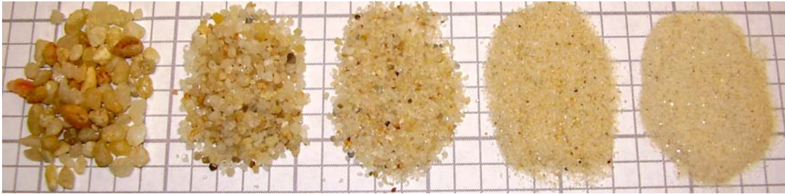
Figure 5-4: Sand from Experiments (Coarsest to Finest)
