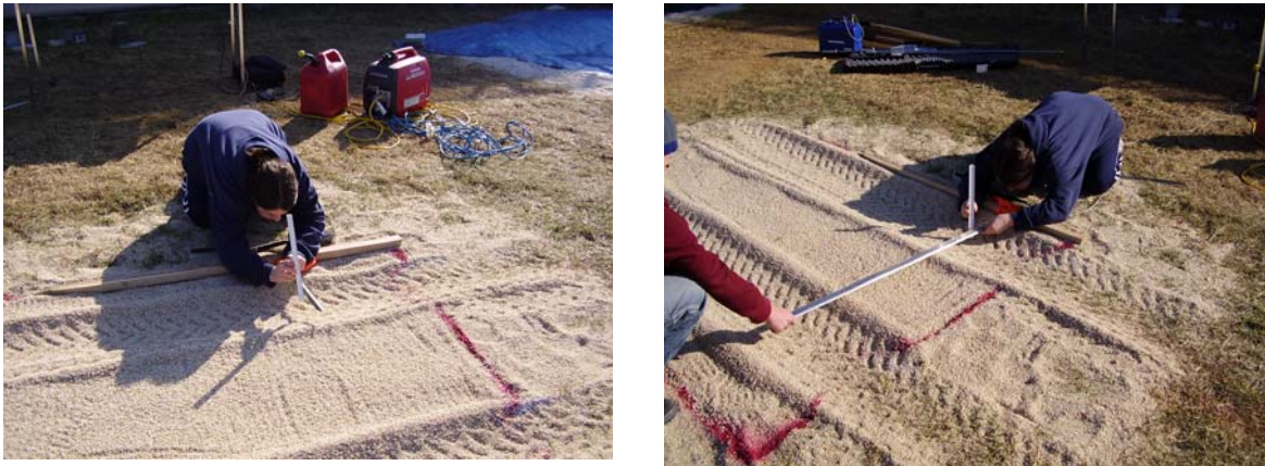
Figure 6-10: Winter 2007 Sinkage Measurement Techniques
