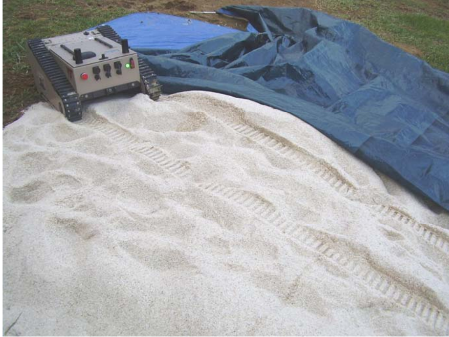
Figure 7-1: MATILDA Successfully Crossing a Large Mound of Loose Sand
