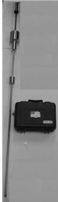
Figure 2-2: Cone Penetrometer with Digital Depth and Pressure Reading
