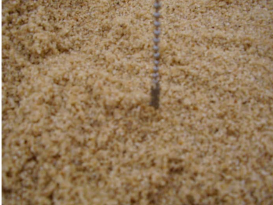
Figure 6-13: Beaded Chain Used to Mark Correct Pressure Sensor Burial Depth in Spring/Summer 2007 Tests
