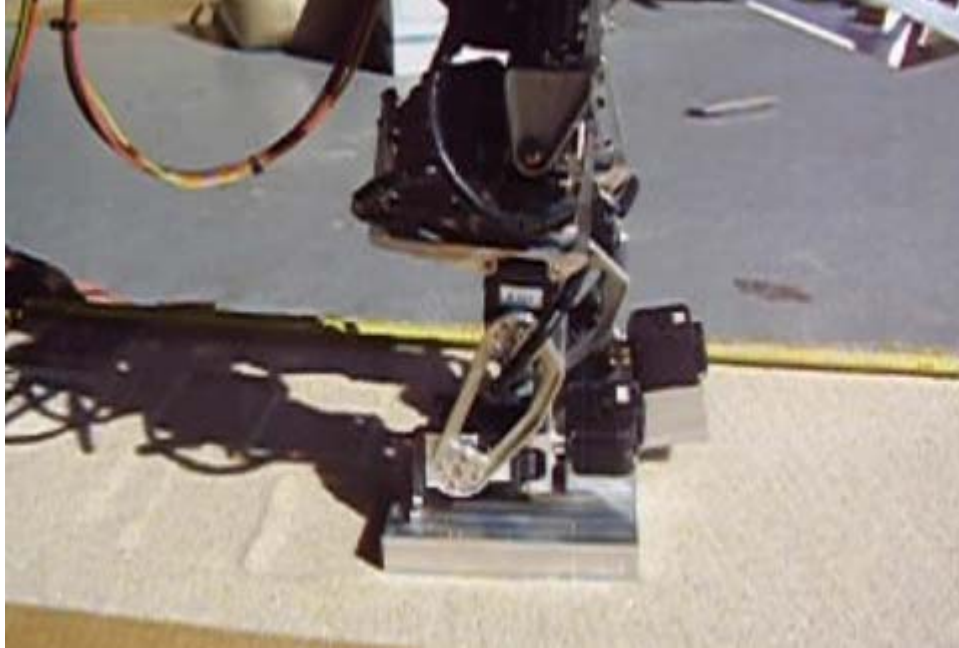
Figure 7-32: DARwIn Right Foot Replaced as Stance Leg, Showing Dragging Marks Behind as Angled Imprints:
