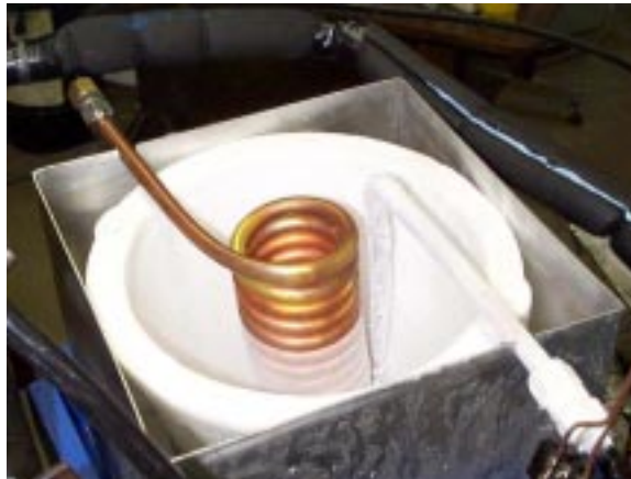
Figure 2.12: Liquid Nitrogen Chiller
