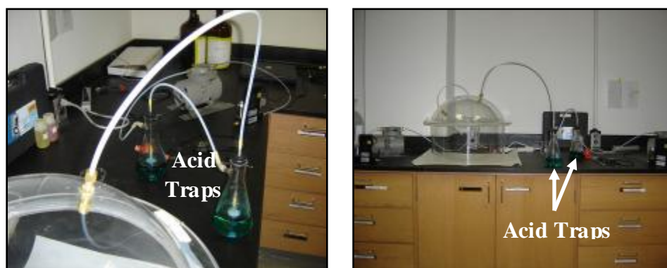
Figure 2.12: Placement of acid traps for ammonia gas sampling
