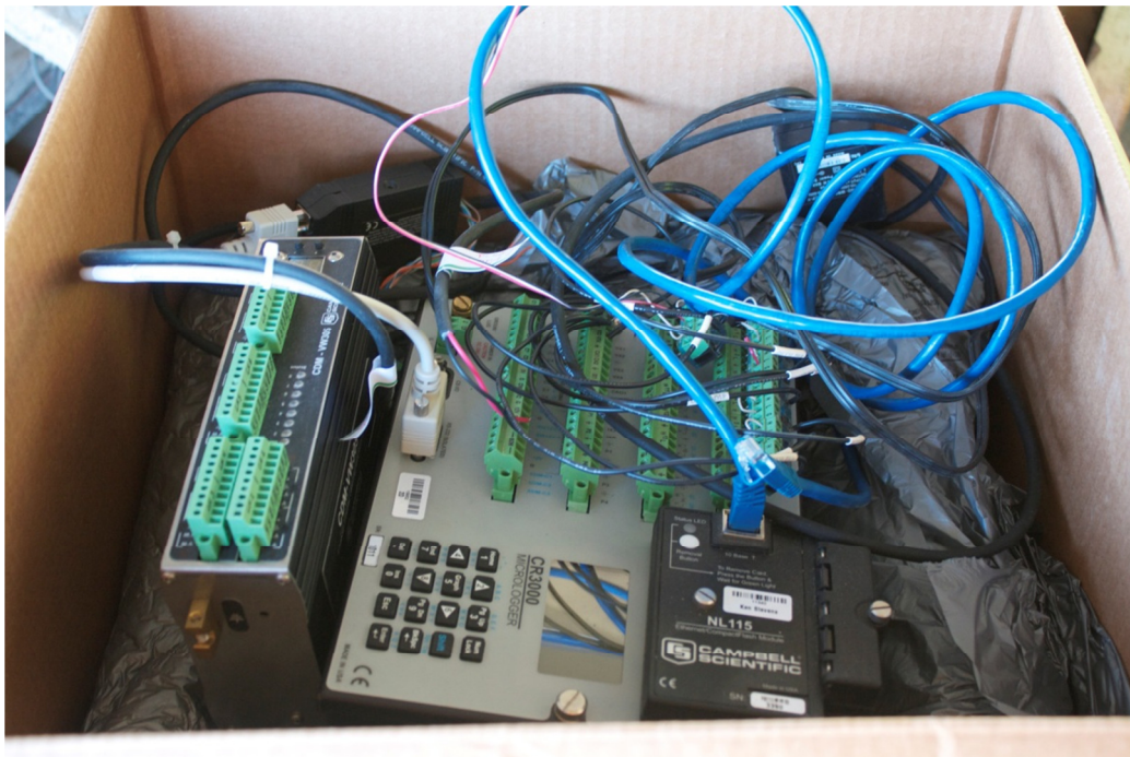
Figure 3-23. Photograph of CR3000 Data Logger
