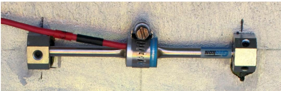
Figure 3-4. Geokon Model 4000 Vibrating Wire Strain Gauge
