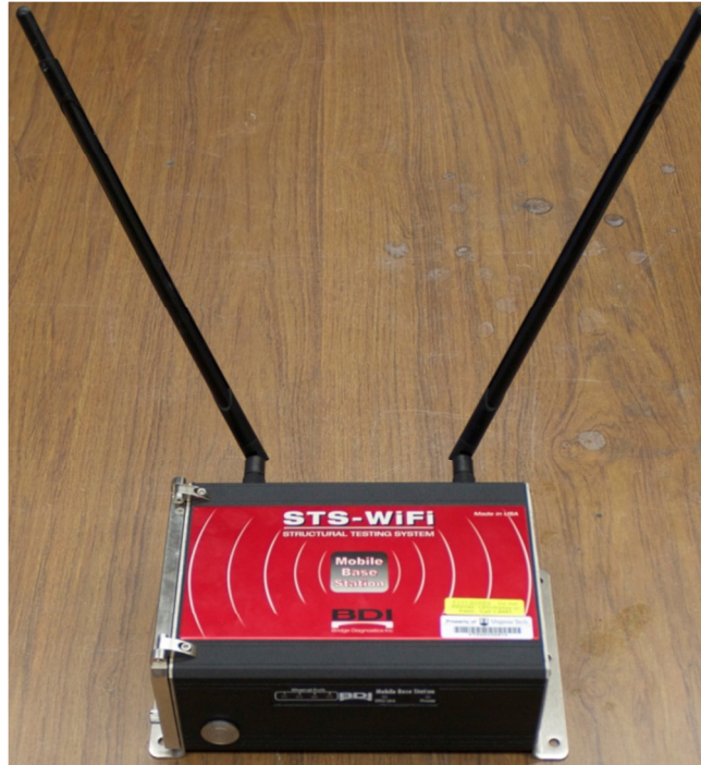
Figure 3-20. Photograph of STS-Wifi Router
