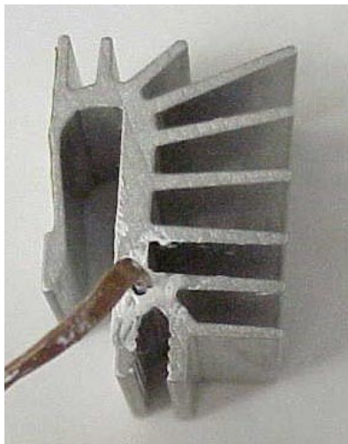
Figure 3.3. Thermocouple placement for the measurement of the device's heat sink temperature.
