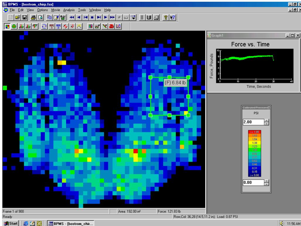
**Figure 3-6. Tekscan BPMS software**
