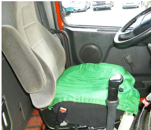
**Figure 3-2. Air-inflated seat cushion mounted on original truck seat**
