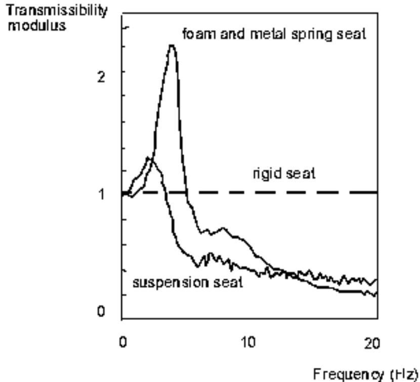
**Figure 2-1. Effect of air-ride suspension, adapted from [3]**
