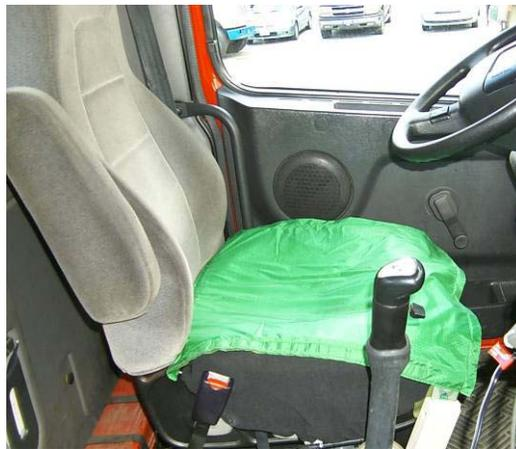
**Figure 3-7. Air-inflated seat cushion mounted on original truck seat**
