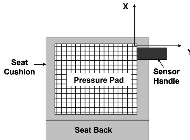
**Figure 3-8. Top view of pressure pad in vehicle coordinate system**
