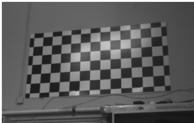
Figure 2.8: Calibration rig used for calibrating the stereo cameras
