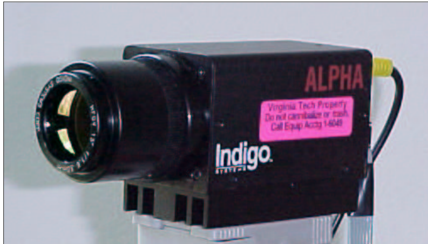
Figure 4.1: Alpha Uncooled Microbolometer Camera by Indigo Systems
