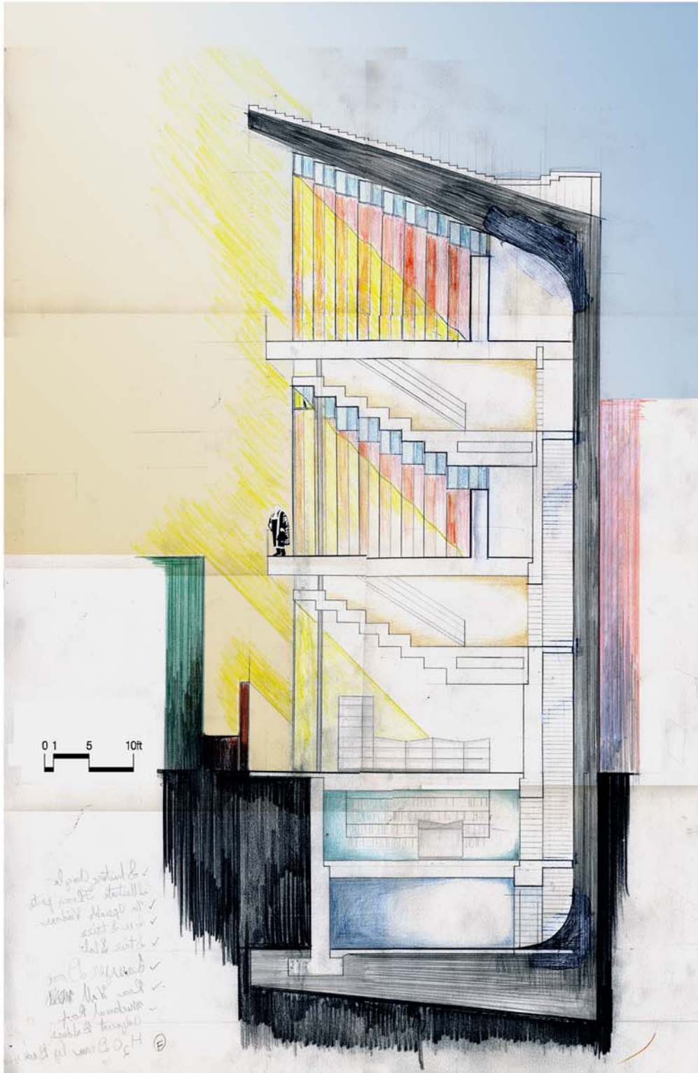
Transverse Building Section cut through the Lawyers Offices, Assistants Levels, Library, File Room, and Mechanical Basement. This section represents the essence of the building and the thesis statement.
