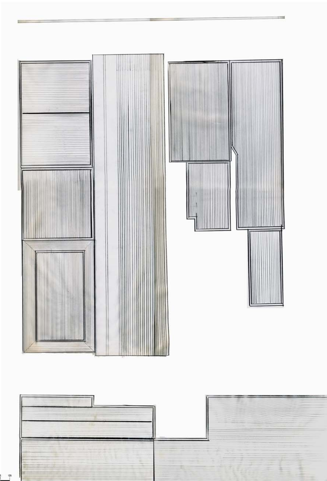
Roof Plan. The roof steps down to a roof fold running the length of the building to collect rain water runoff and direct it toward the back of the site.
