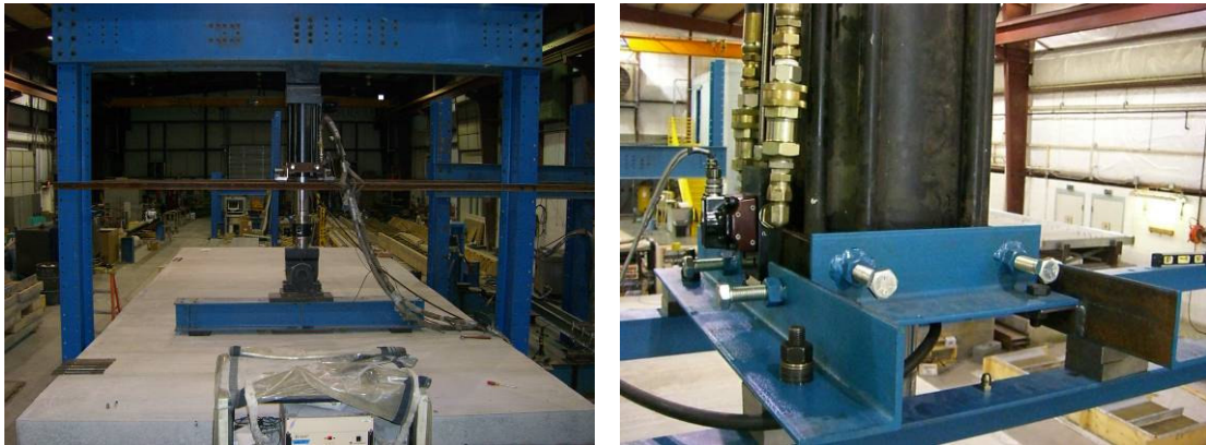
Figure 3.20: Fatigue testing setup
