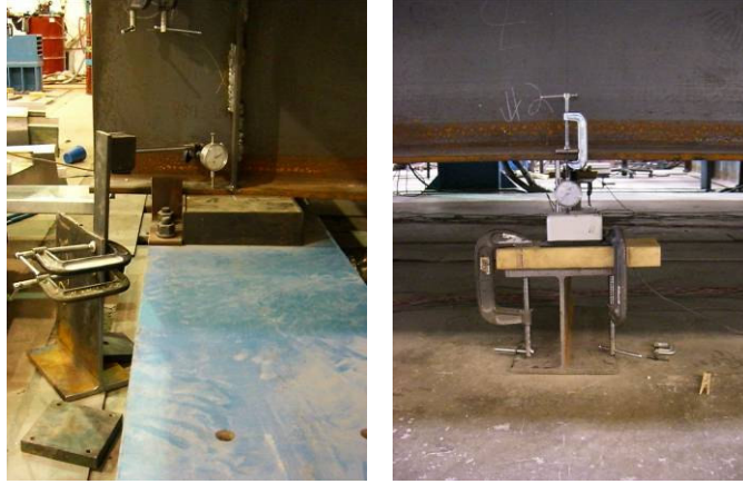
Figure 3.15: Vertical deflection sensors (a) support dial gauge placement (b) in-span dial gauge and wire pot placement
