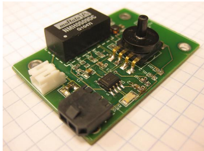
Figure 3-9. Simulation PCB after populating the components. Photo by author, 2012.
