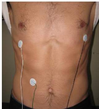
Figure 3-23. ECG lead locations during human testing. Photo by author, 2012.
