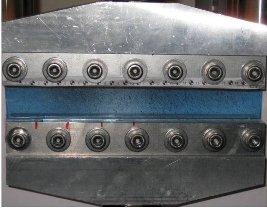
Figure 4-28: Constrained tension fracture sample with speckle pattern
