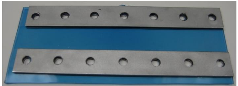
Figure 4-11: Hydrogel sheet with attached aluminum reinforcement bars
