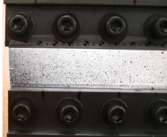
Figure 4-29: Close up of speckle pattern on Hydrogel A
