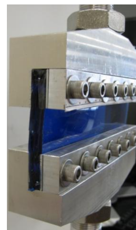
Figure 4-24: Side view of four times thicker constrained tension sample
