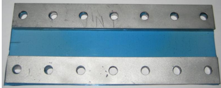
Figure 4-12: Finished constrained tension fracture sample (Hydrogel A)
