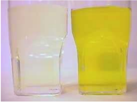
Figure 5-2: Color difference in water from 0.5 mg/L silica container (left) and 50 mg/L silica container (right) at 20 0 C.
