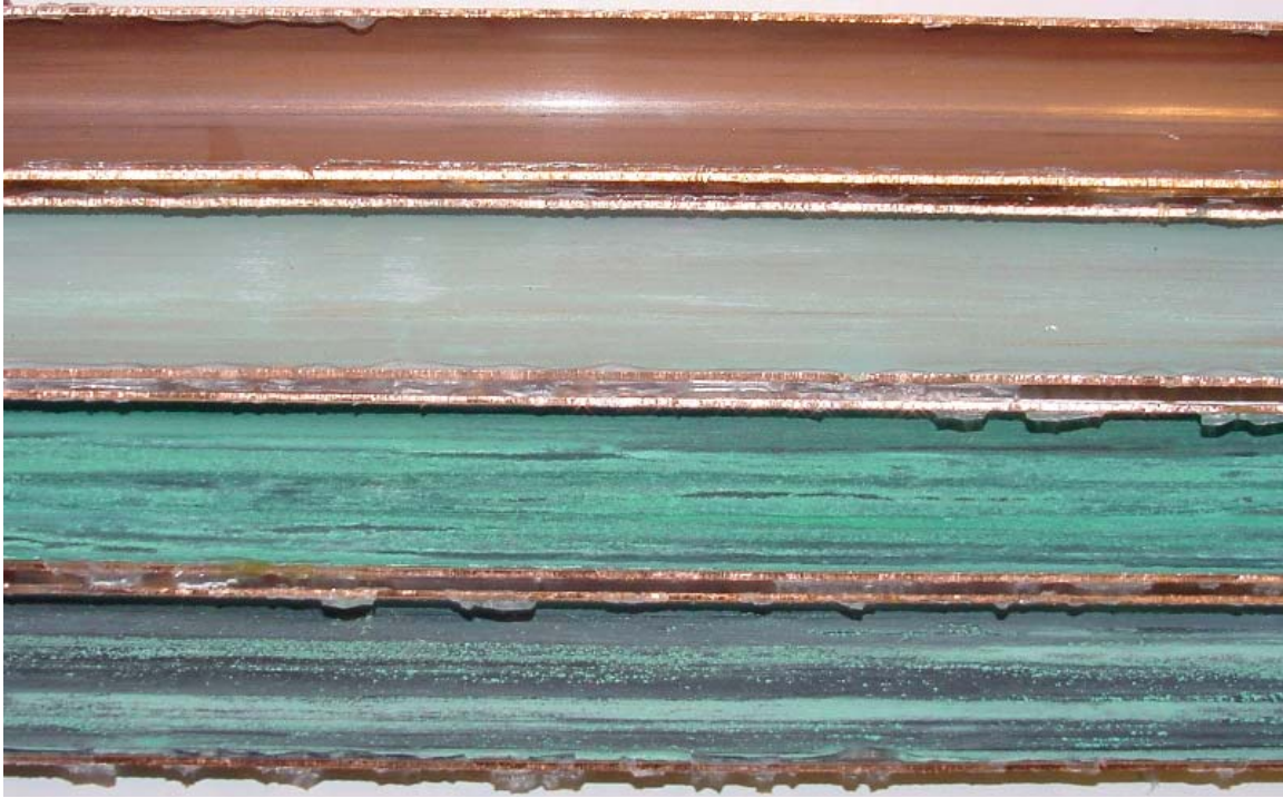
Figure 2-11: Dried copper pipe samples at the end of the experiment. From top to bottom: Control, 1 mg/L Al, 3 mg/L Cl 2 , 1 mg/L Al plus 3 mg/L Cl 2 .
