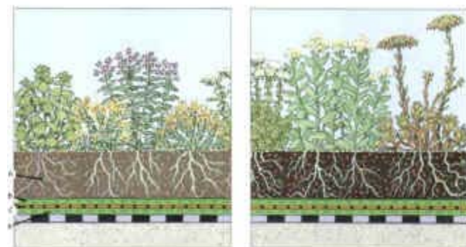
Simple Plant Communities: Height: 2 – 3 inches A – “Optima-Kennkorper” Extensive Soil Substrate B – Insulation Layer C – Root Barrier Course D – Waterproof Membrane Protective Barrier
