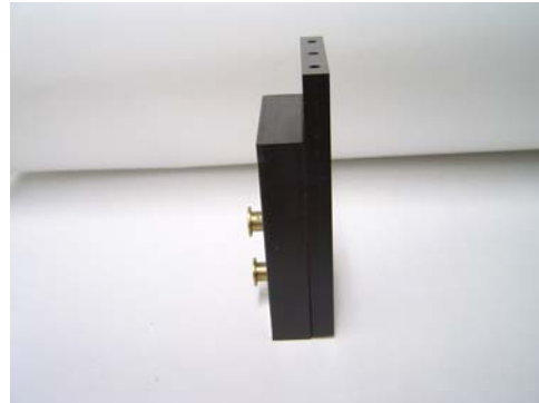
Figure 3. Second generation 2-piece slide holder. Contact surface area \sim 77 \text{ cm}^2 .
