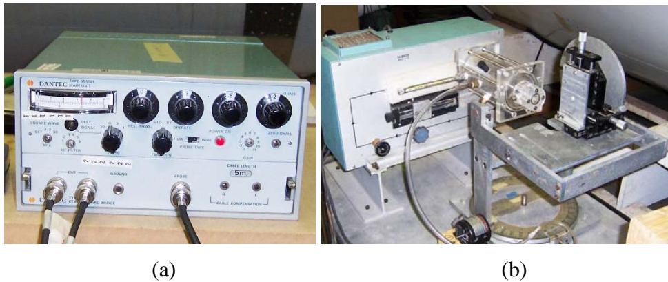
Figure 2- 6 : a) Power supply used to power and regulate the hot wire anemometer b) TSI Calibrator model 1125 used to calibrate the output of the hot wire anemometer.
