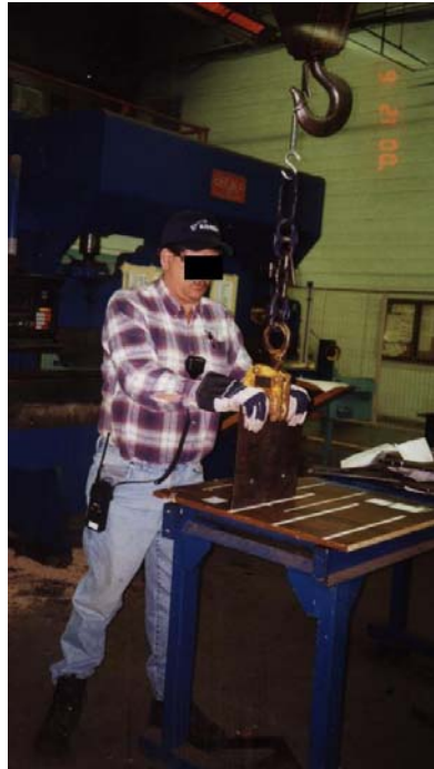
Figure 4.3: One person with a spring-equipped overhead crane
