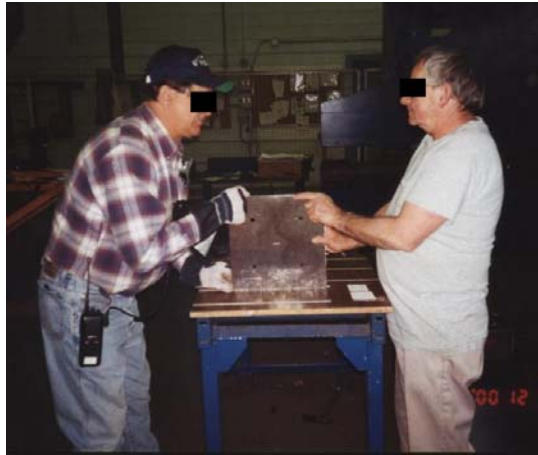
Figure 4.1: Two-person team without an overhead crane
