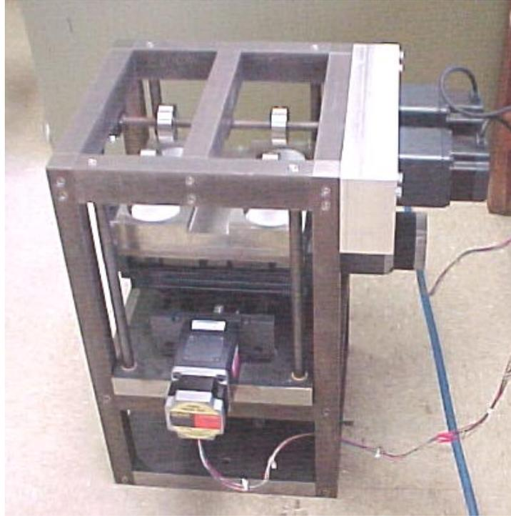
**Figure 4-3. Photograph of the completely assembled device. The frame, the table support, and the vertical guide rods can be seen here, as well as the placement of the bolts, which fastens the components together.**
