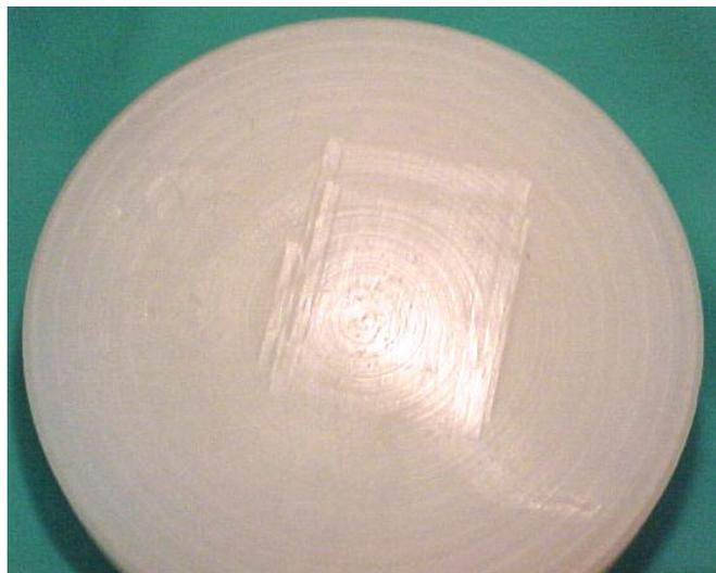
**Figure 5-5. The worn UHMWPE block after 50,000 cycles of testing. The wear track can be seen as a shiny rectangle on the material's surface.**
