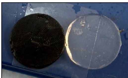
Figure 3.2. Tissue phantoms shown here, 0.1 mg/ml MWNT phantom (left) and non-NT phantom (right).
