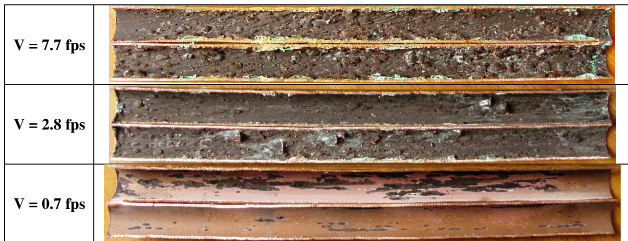
Figure 1 – 9: Effects of Velocity on Scale and Tubercle Formation on the Third Pipe in Flow for ¾” Diameter Tube
