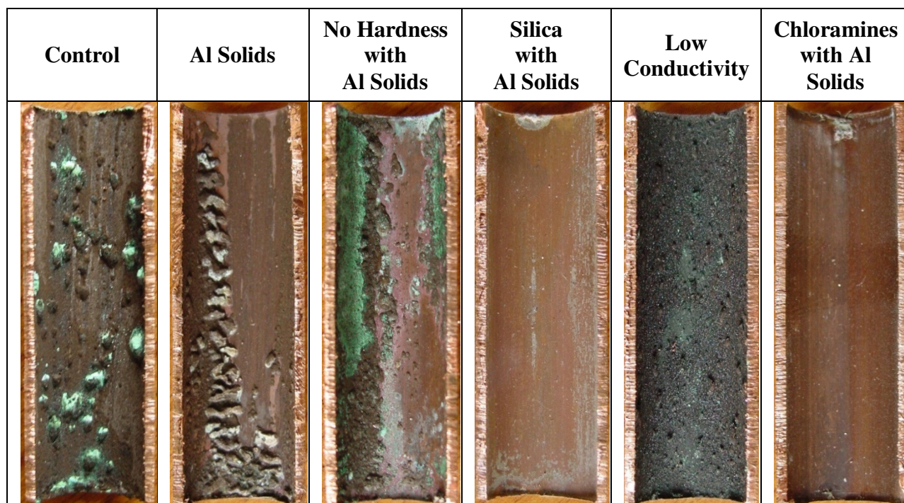
Figure 2 – 5: Scale Formation on Copper Coupons
