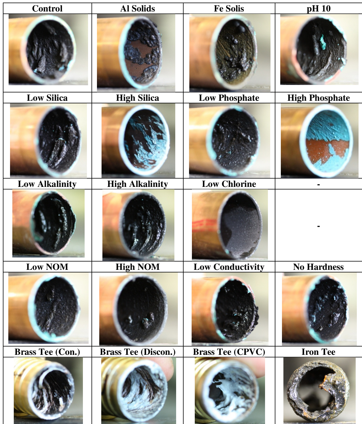
Figure A – 4: Corrosion Scale in Tees After 4 Months
