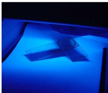
Step 5: Cure glue with 365 nm UV lamp for 5 minutes.
