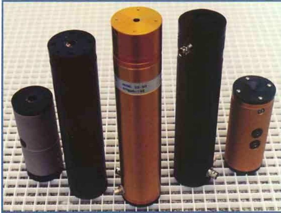
**Figure 1-1: Some crystal based EO modulators.**
