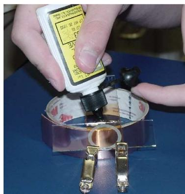
Step 4: Deposit optical glue at the interface and let seep through to spacer.
