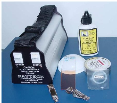
Step 1: Required equipment/hardware for sample preparation.
