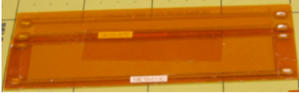
Figure 7.13: 85x15mm MFC element with 85x3mm MFC for sensing.
