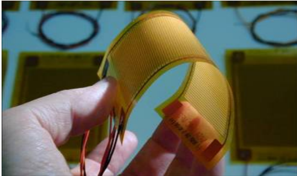
Figure 1.4: Sample MFC patch. Image credit Smart Materials Corp. ( www.smart-material.com )
