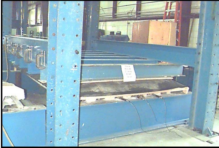
Figure 4.3. 3 Full-Scale Slab Test Set Up
