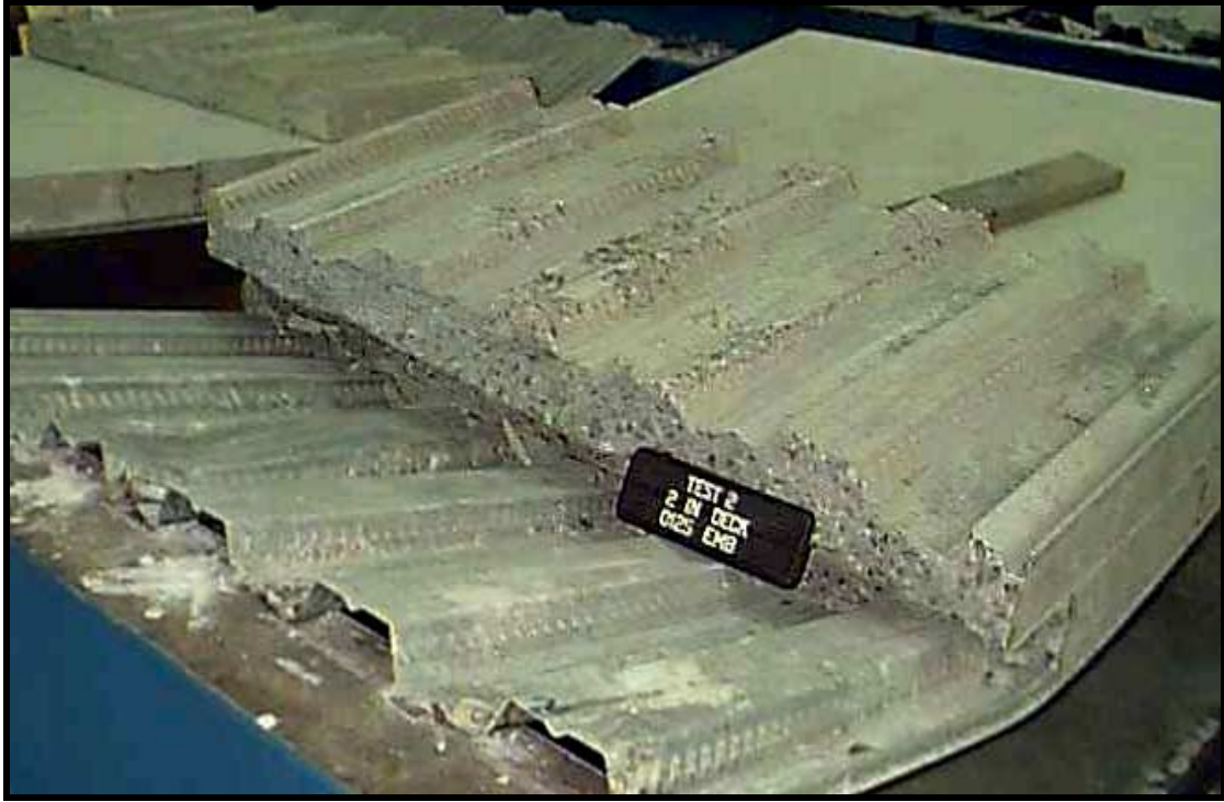
Figure 4.5. 2 Honeycombing of the 2-0.125i-a Specimen
