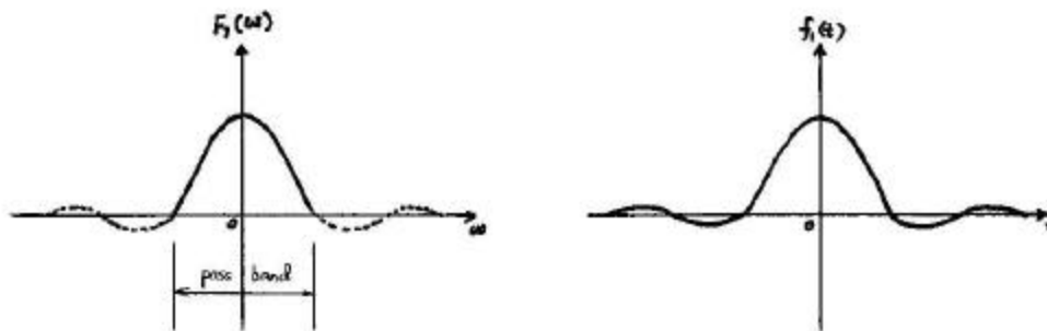
Figure 2.6(a) small bandwidth and reconstructed signal
