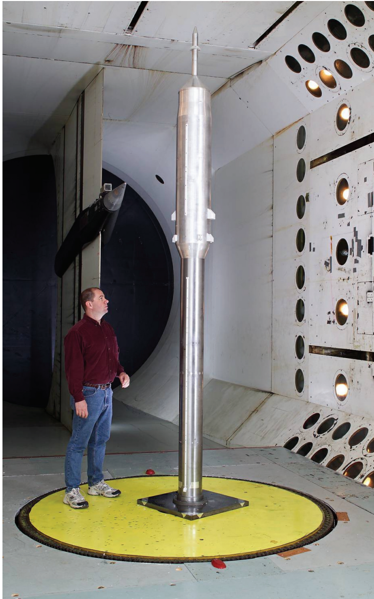
Figure 34. GWL Checkout Model installed in TDT. (Photo Credit: NASA, used with permission)
