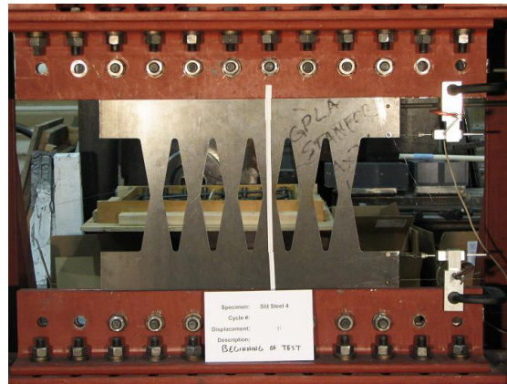
Figure 11: Panel with butterfly fuse [from (Borchers, Peña, Krawinkler, and Deierlein 2010)]
