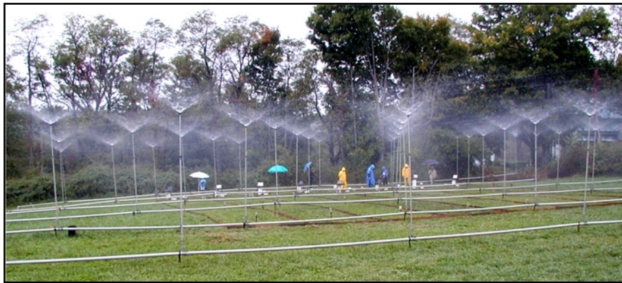
Figure 8. The portable rainfall simulator rains on the transport plots
