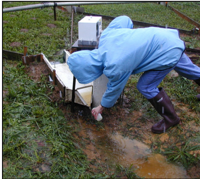
Figure 9. Becky Zeckoski, a research associate at Virginia Tech, collects a grab sample from the flume located at the bottom of a transport plot.
