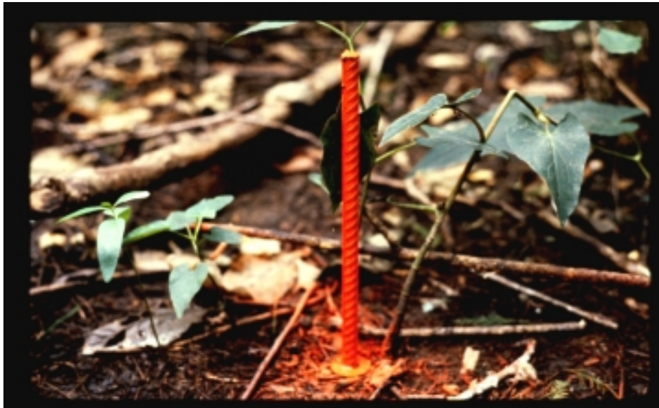
FIGURE 12. Sediment rod used in experiment in a tupelo-baldcypress forested wetland in the Mobile-Tensaw River Delta of southwestern Alabama.
