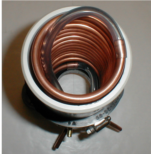
Figure 4.20 Interior view of cooling jacket
