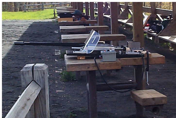
Figure 5.5 Gun recoil demonstrator at firing range
