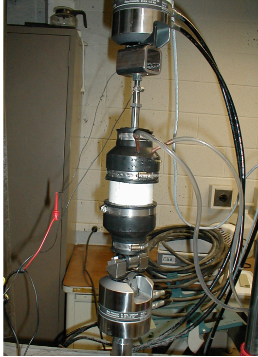
Figure 4.19 Ford Expedition MR damper in the MTS machine (cooling jacket installed)
